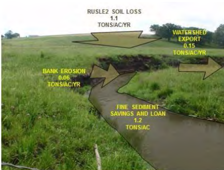
Figure 5. Example of a historical sediment budget, in tonnes per year, for a steep forested watershed in the upper Great Lakes (Fitzpatrick et al., 1999; Fitzpatrick and Knox, 2000). Bluff erosion was identified as a major source of sediment that was causing downstream sedimentation problems in fish spawning riffles.
