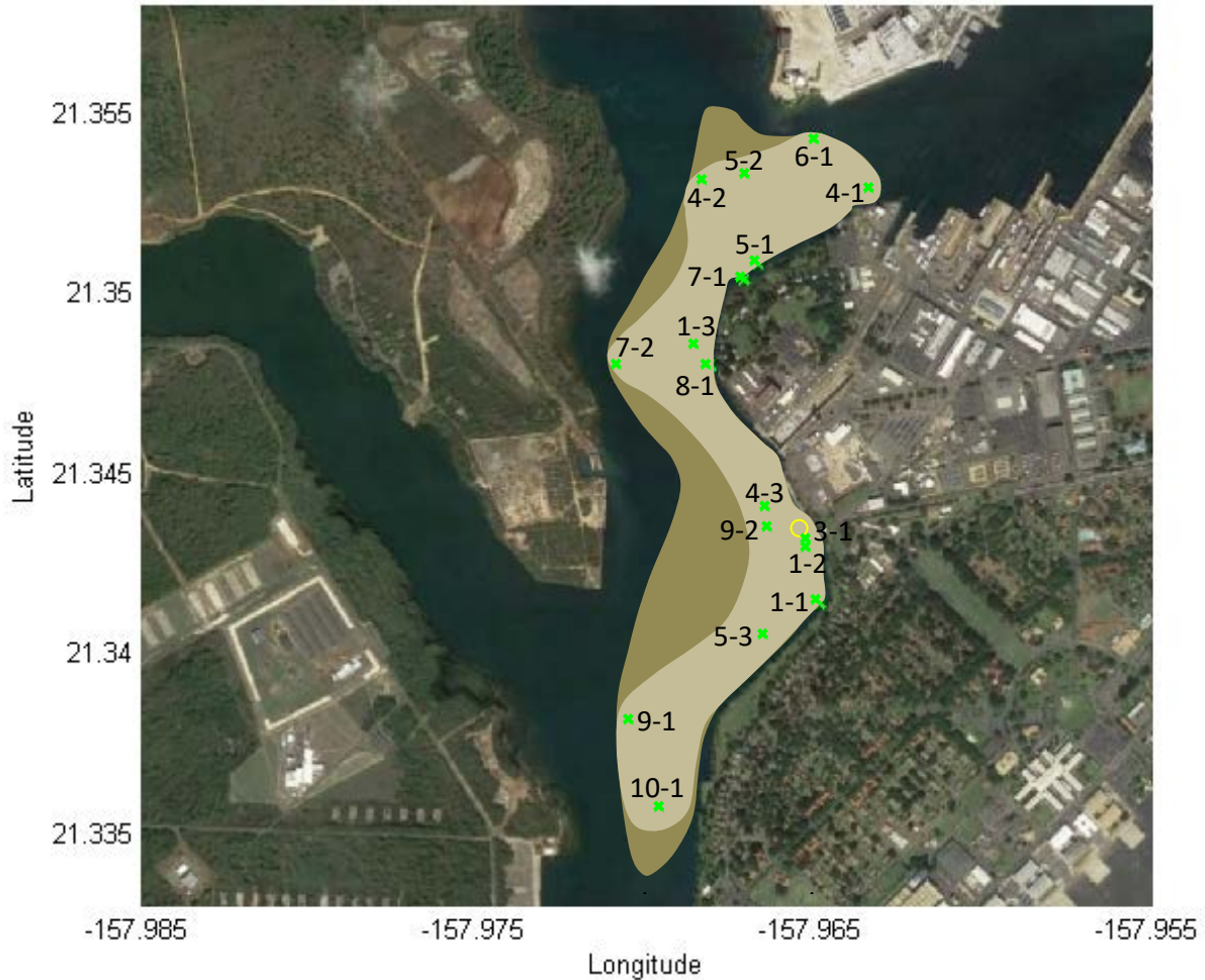
Figure 28. Deposition Footprint with Connectivity to the Stormwater Discharge Outfall Near Oscar Pier. The Light Shaded Area Indicates the Area Encompassed by the Actual Bottom Contacts for the Target 34 mm/min (silt) Settling Rate Particles. The Darker Shaded Area Encompasses the Trajectories and Bottom Contacts and is Representative of the Potential Deposition of Particles Sinking at \leq 34 mm/min (Silts and Sands). The Green x's Are the Actual Bottom Contact Locations.
