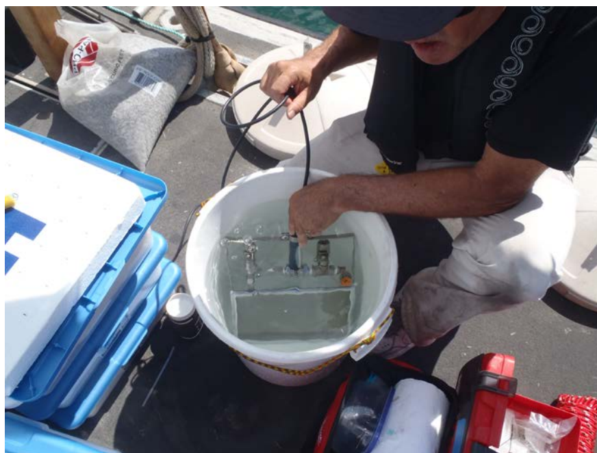
Figure 15. Purging the Pressure Plate on the SeDep Prior to Deployment at the Oscar Pier Site.
