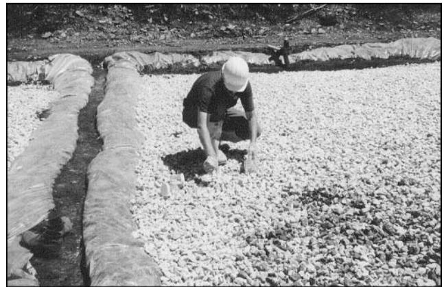
Figure 6—Mesocosm after placement of broken limestone ballast in an identical configuration with the right-of-way crossing the Des Plaines River wetland.
