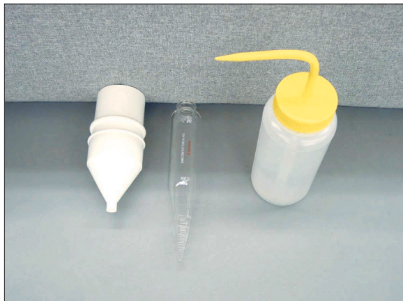
Figure 1. Apparatus used by the petroleum industry for determining sand content by volume
