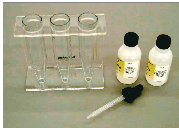
Figure 2. Test kit apparatus for determining sand, silt, and clay percentages by volume
