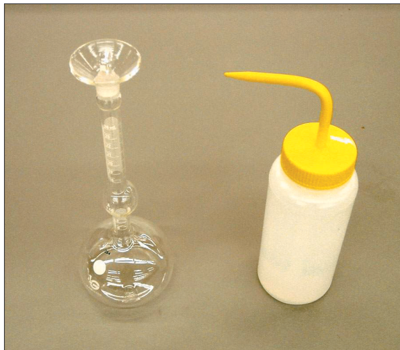
Figure 6. Specific gravity measurement with a Le Chatelier flask
