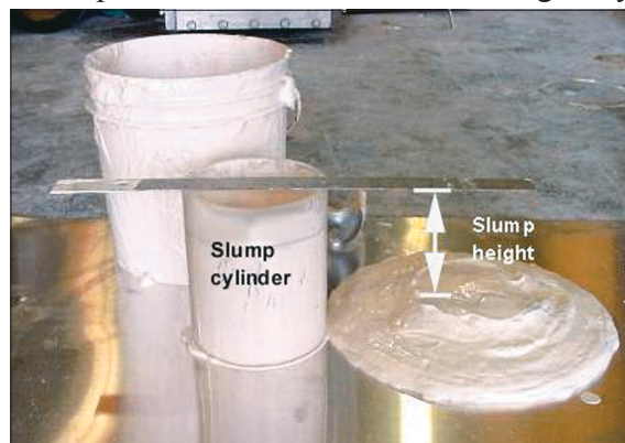
Figure 10. Dredged material slump test
