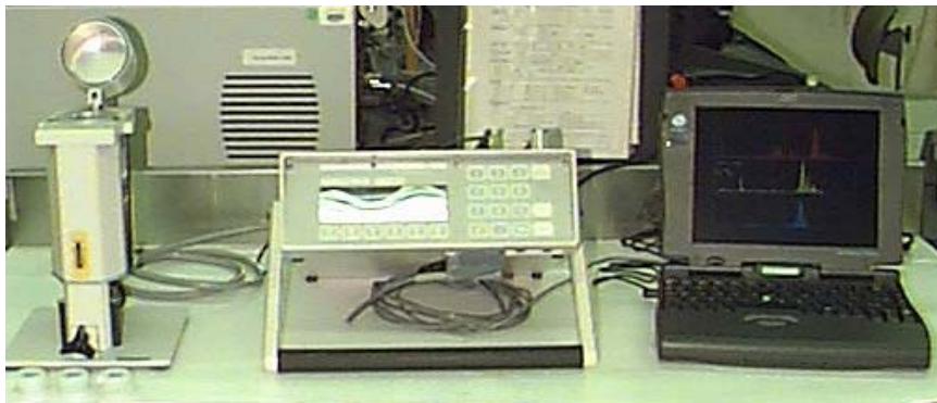
Figure 7. Spectrace 9000 FPXRF (probe, multi-channel analyzer, laptop computer).
