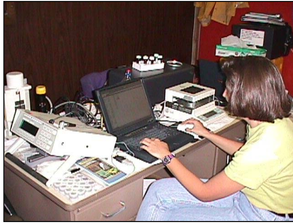
Figure 8. On site analysis by FPXRF, Demo #2.
