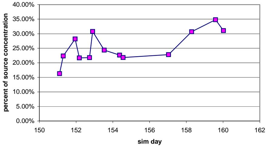
Figure 24. Bromide recycling at biotreatment wells during tracer test. Note: The figures show the percent of source concentration that instantaneously appears at the non-injection screen.
