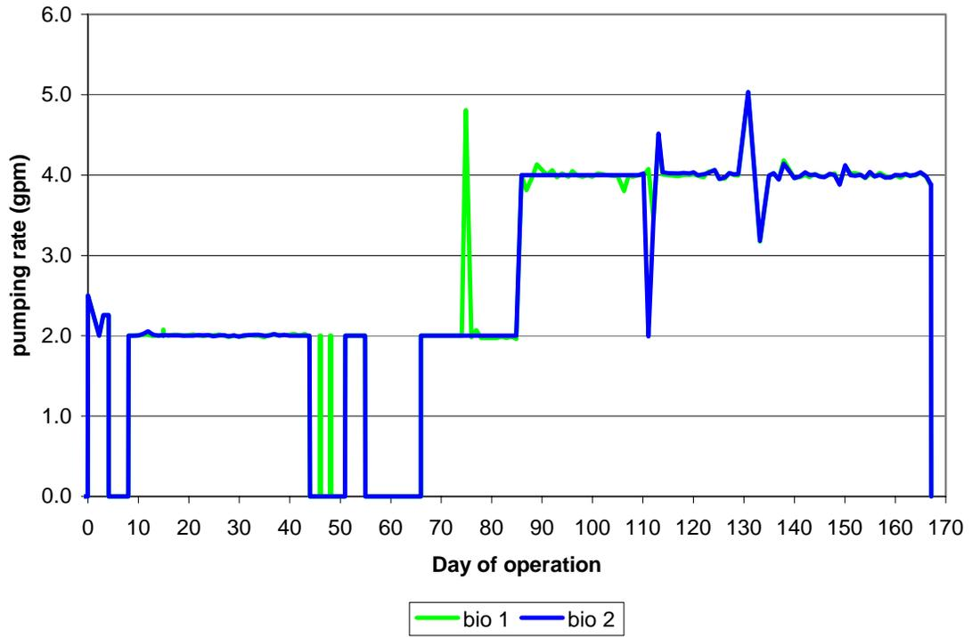
Figure 7. Measured pumping rates at biotreatment wells.
