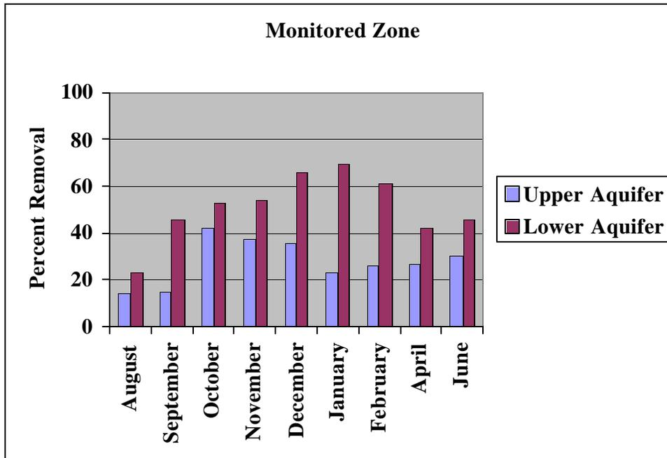
Figure C1. TCE percentage removals compared with initial values at start of in upper and lower aquifers with time for treatment zone and monitored zone.
