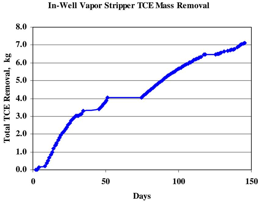
Figure 6. Mass of TCE removed by vapor stripping well, calculated as the difference between integrated masses through upper and lower wellscreens.
