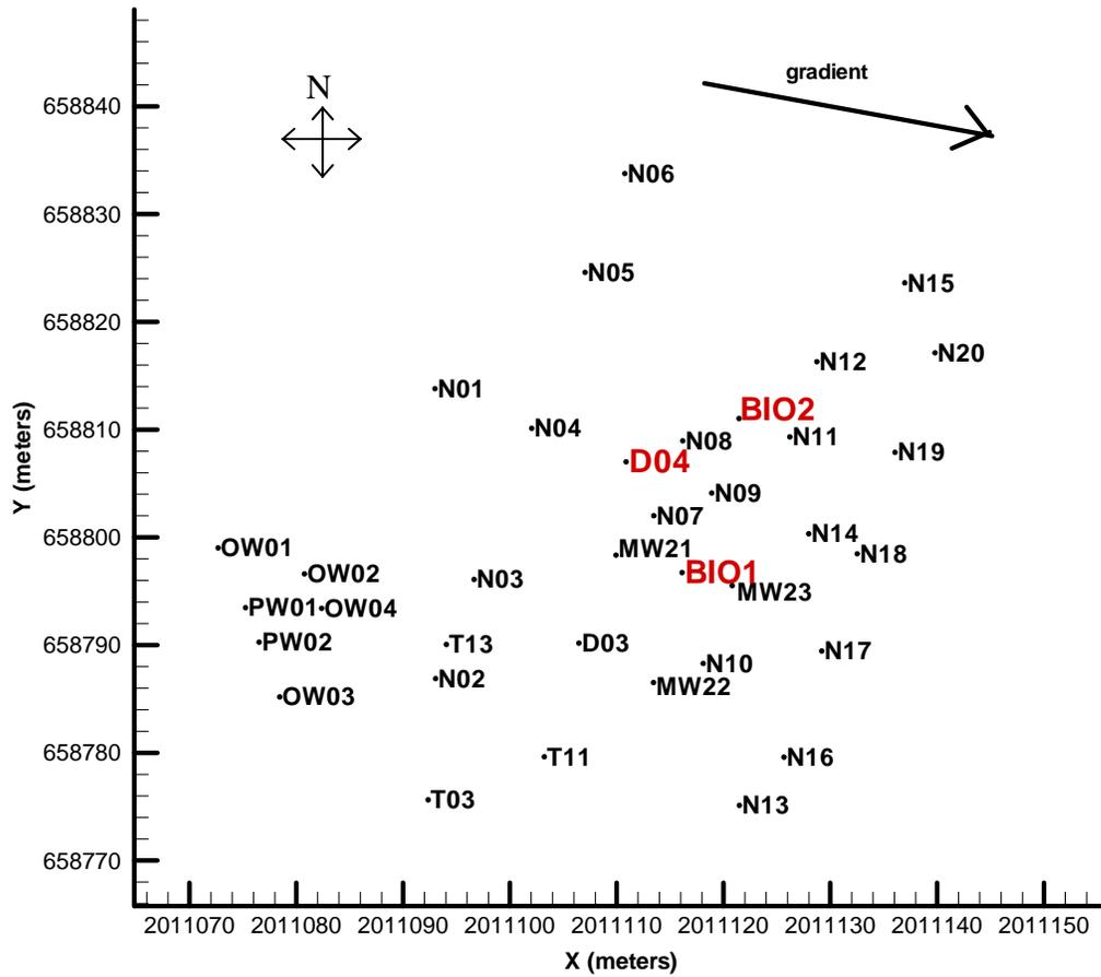
Figure 2. Plan view showing locations of the BEHIVS in-well vapor stripper (D04), the two biotreatment wells (BIO1 and BIO2), and monitoring wells.
