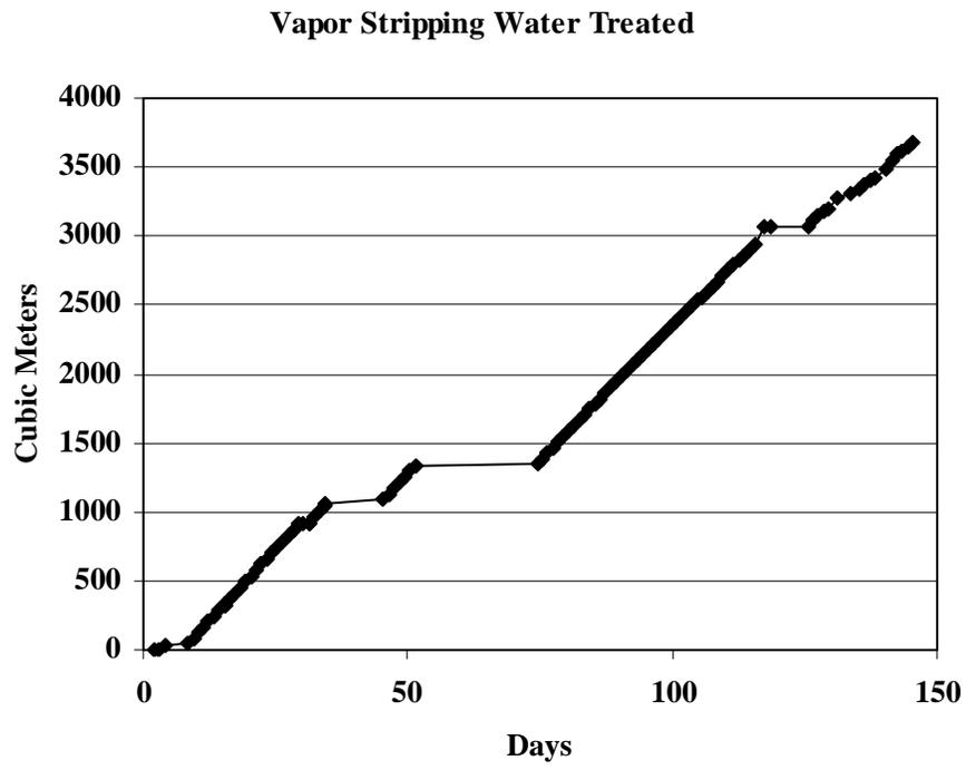
Figure 4. Total water treated by vapor stripping well.
