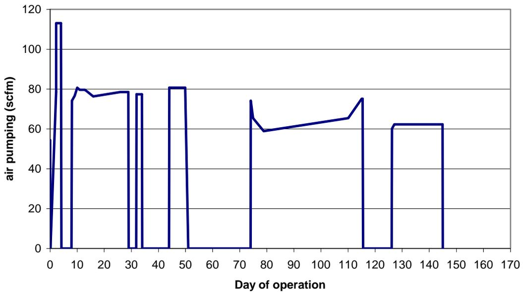
Figure 3. Operation of In-Well Vapor Stripper, water flowrates and air pumping rates.
