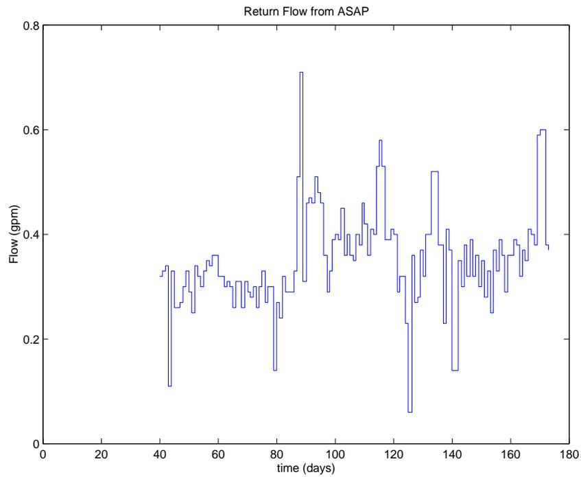
Figure 21. Sampling return water flow volume. Note: This water is injected into the biotreatment wells until January 9, 2002, at which point it is returned via the upper screen of the IWVS.
