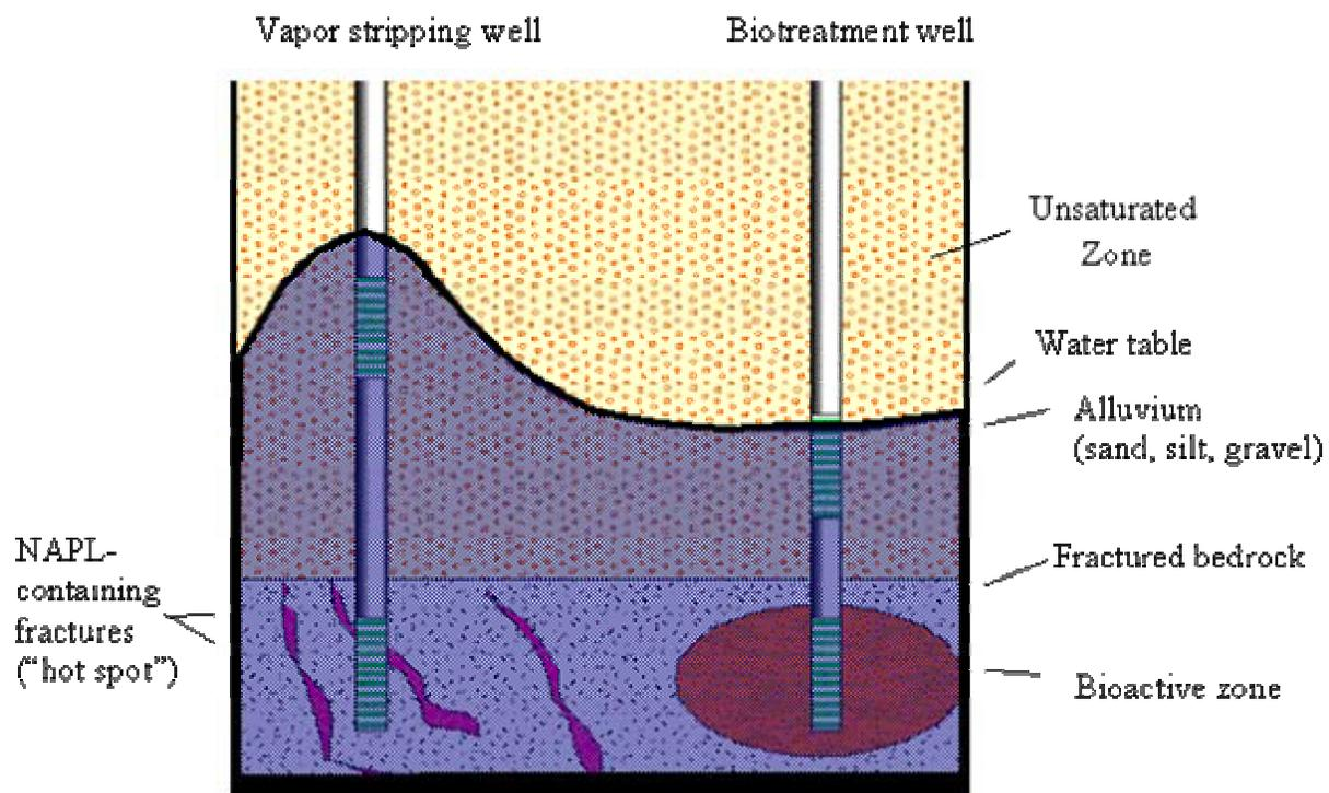
Figure 1. Schematic plan view of the BEHIVS treatment system.
