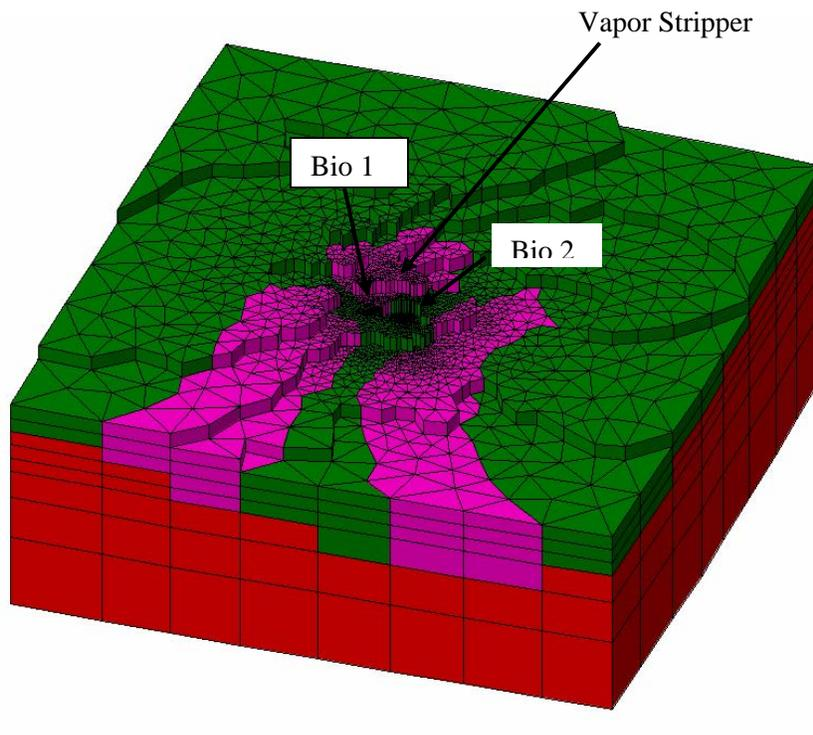
Figure 17. Weathered bedrock elevation (in meters) in BEHIVS model. Note: The green material is the weathered bedrock and red is the competent bedrock below. The pink material is the low conductivity zone within the lower aquifer.
