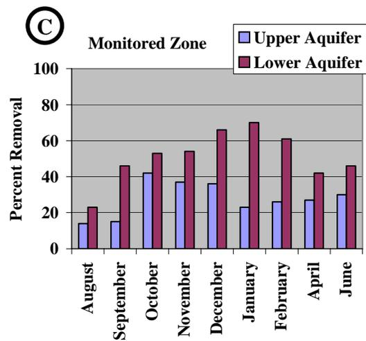
Figure 12. Percentage of TCE removal by BEHIVS treatment in the upper and lower portions of the aquifer at Edwards Air Force Base. Note: Figures showing (A) map of treatment zone, (B) monthly percent removal in the treatment zone, and (C) monthly percent removal in the monitored zone.
