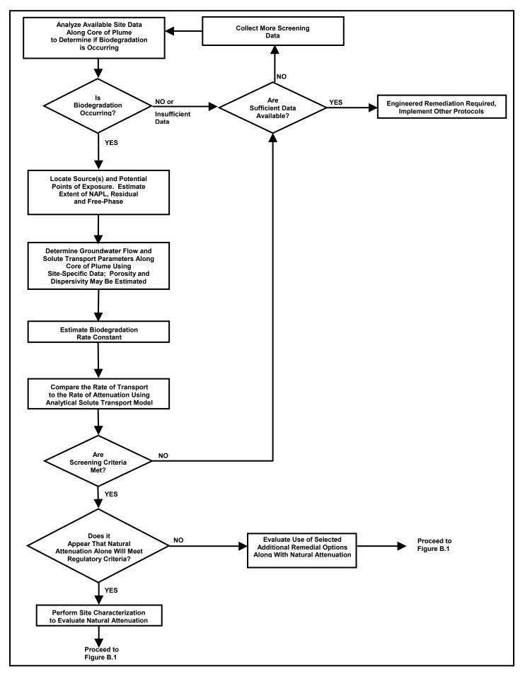
Figure B.2 Initial screening process flow
