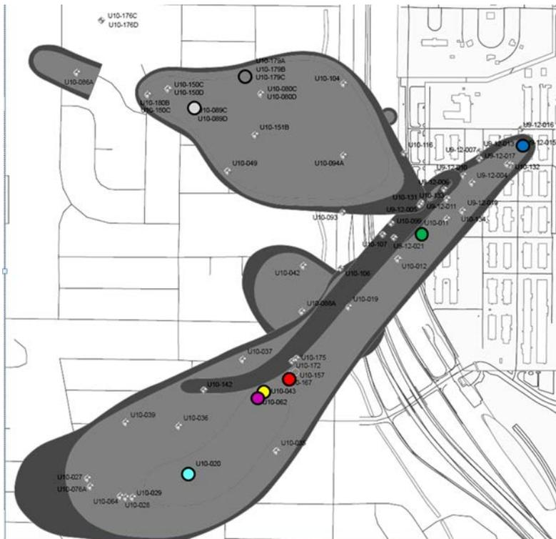
**Figure A-4.** Map of the wells with TCE  $\delta^{13}C$  and  $\delta^{37}Cl$  potentially similar to the original solvent signatures indicated in **Figure A-3**. Well location colors are those presented in **Figure A-3**.
