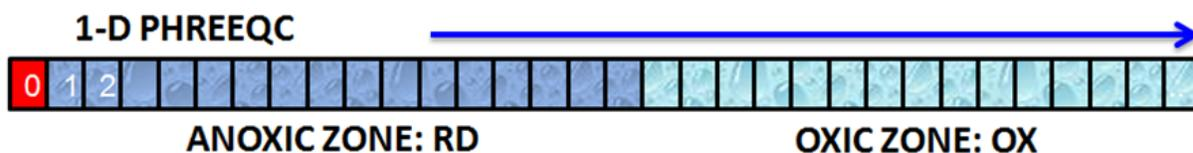
**Figure 4-9.** Model setup (1-D PHREEQC) for incomplete dechlorination under anoxic conditions (RD= reductive dechlorination) resulting in a stall of VC with potential an (aerobic) oxidation (OX) further downgradient.
