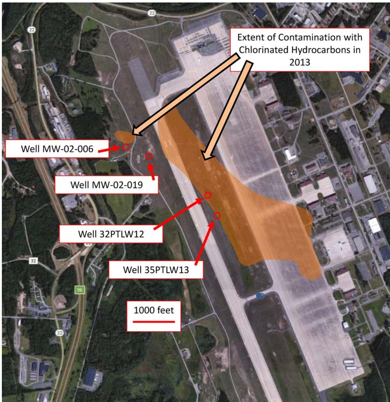
**Figure 4.2.4. Sampling Locations for EAPs, qPCR, and <sup>14</sup>C-labeled TCE Assay were Well MW-02-006, Well MW-2-019, Well 32PLTW12 and Well 35PLT13.**
