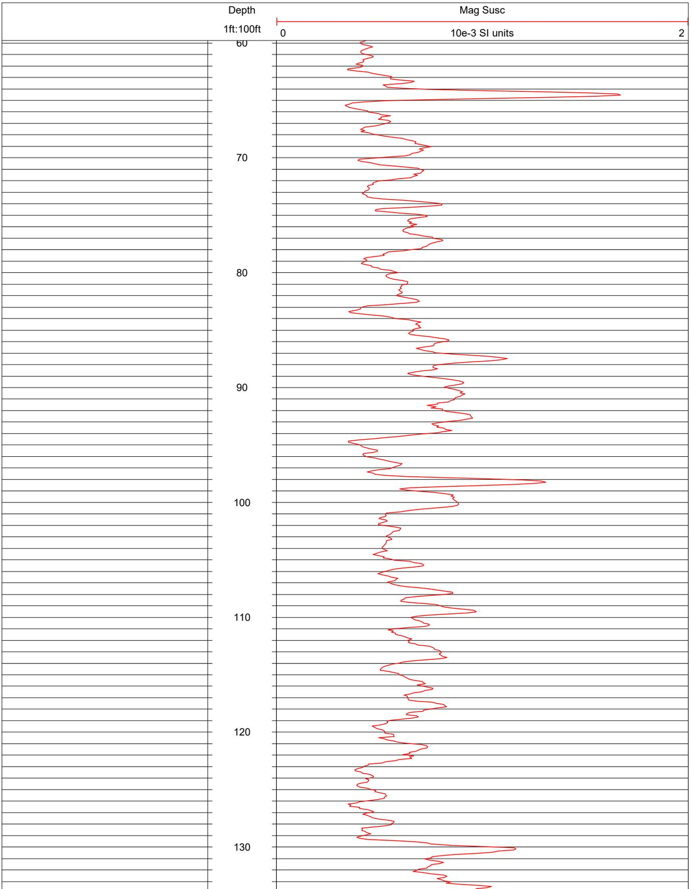
MASS MAGNETIC SUSCEPTIBILITY DATA FROM THE SONDE FOR HILL AFB-OU10, HILL AFB, UTAH
