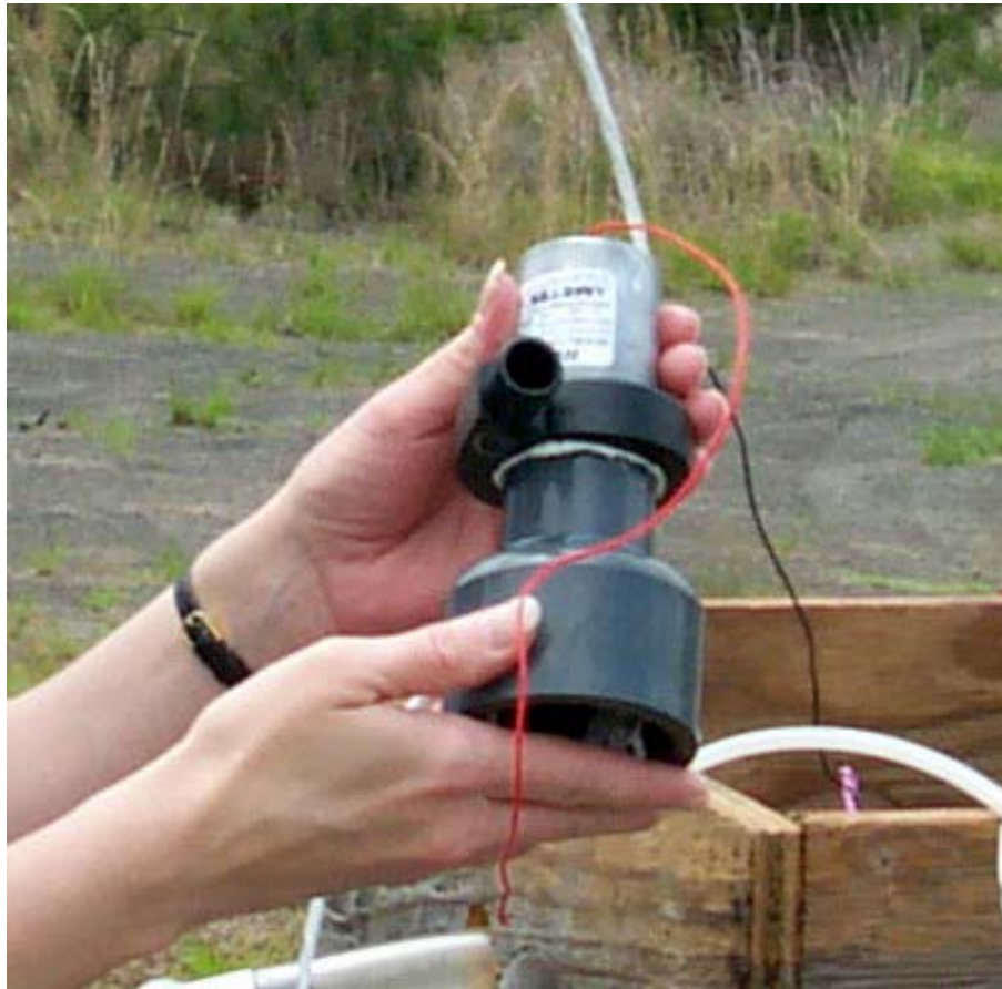
Figure A-11. Microblower Used to Enhance Soil Vapor Extraction ( http://www.srs.gov/general/enviro/erd/technology/Pages/h10p.html )
