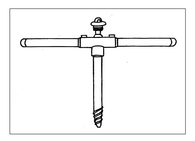
Note that, although not clearly illustrated above, the borer bit is a hollow tube threaded at the boring end. (Source: Bonham, C.D., "Measurements for terrestrial vegetation," John Wiley & Sons, New York, NY, 1989, p. 45.)
