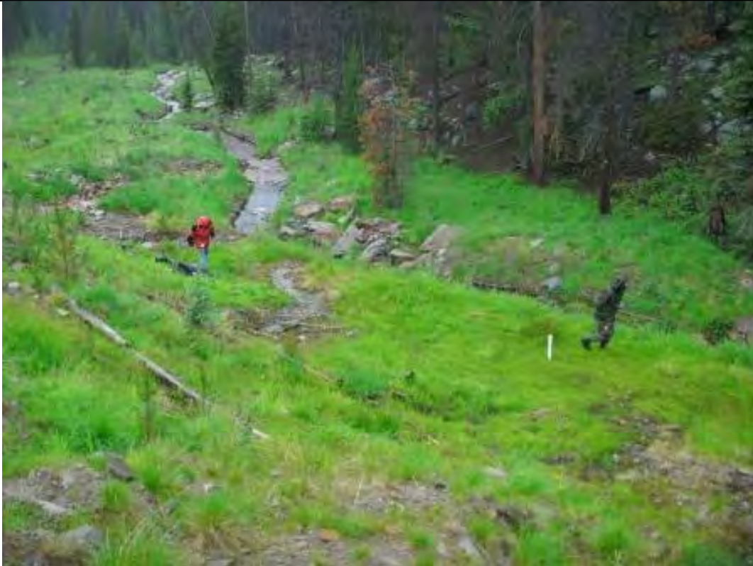
Running seismic refraction lines along Jill Creek floodplain
