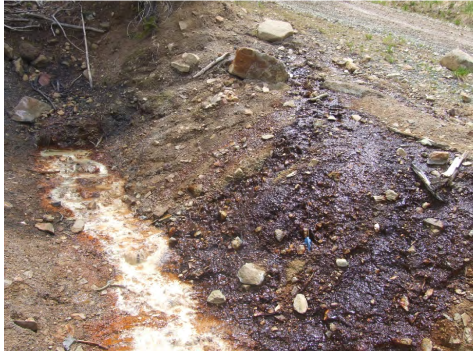
PHOTOGRAPH 2-1. Acidic Discharge from Collapsed Adit Section
