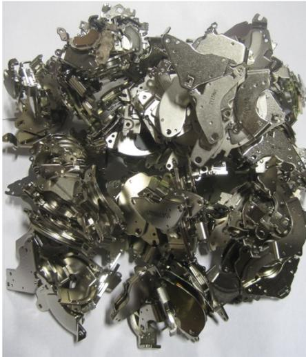
Hard drive Nd-Fe-B scrap magnets with bracket assembly
