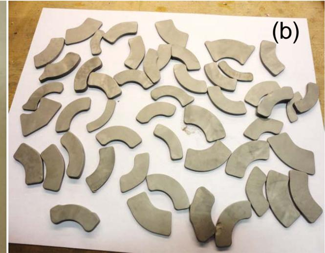
EEC's proprietary approach to make Ni/Cu coating free Nd-Fe-B magnets for reuse/recycle
