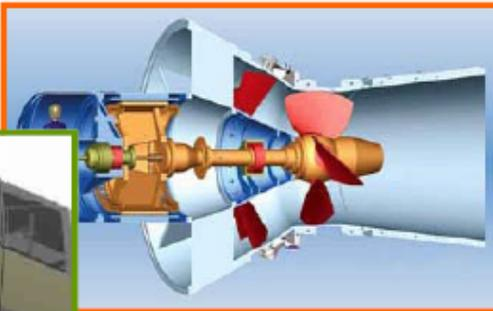
PM hydroelectric turbine generators eliminate need for gearboxes
