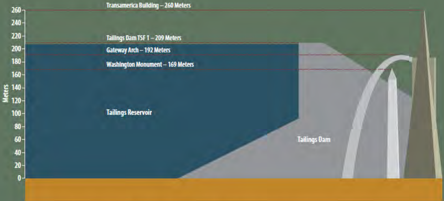
Height of the Dam at TSF 1 In the Pebble 2.0 and Pebble 6.5 Scenarios, Relative to U.S. Landmarks
