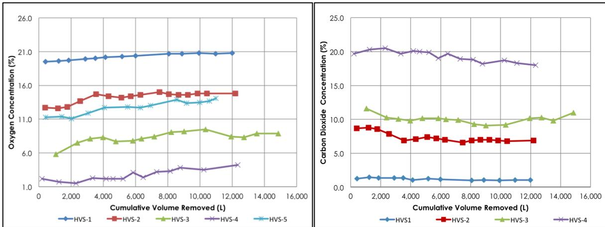
Figure 3: Example data for O<sub>2</sub> and CO<sub>2</sub> as a function of volume purged (McAlary, 2016)
