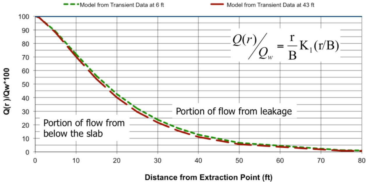
Figure 8: Relative proportions of flow from above and below the floor as a function of distance from the suction point (McAlary et al., 2011)
