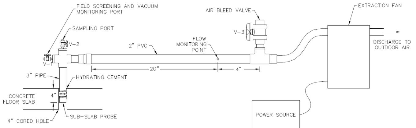
**Figure 1: Schematic diagram of HVS test equipment (Courtesy of Geosyntec)**
