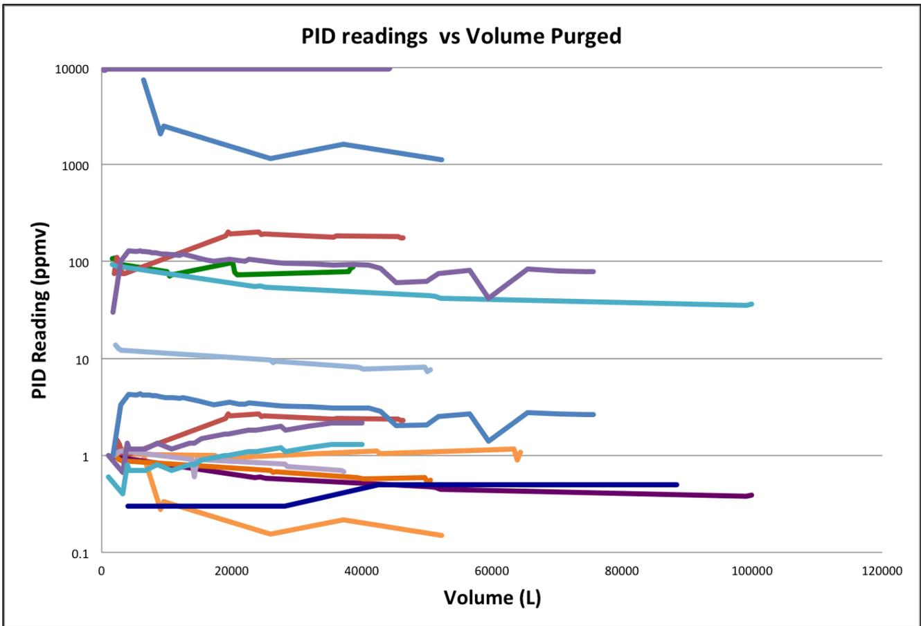
Figure 2: Typical PID readings from HVS tests (Courtesy of Geosyntec)
