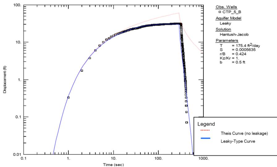
**Figure 7: Example of mathematical model fitting to the transient vacuum response data (McAlary et al., 2011)**
