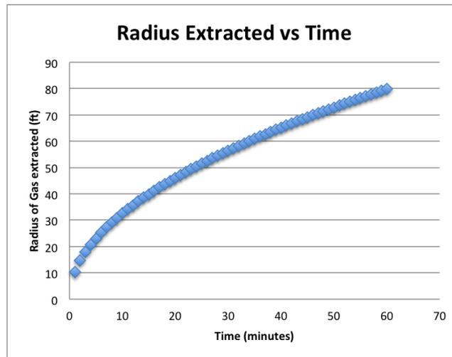
**Figure 4: Approximate radius from which gas would be extracted as a function of time during an HVS test at 50 scfm (with a 6-inch gravel layer of 30% porosity below a competent slab) (Courtesy of Geosyntec)**
