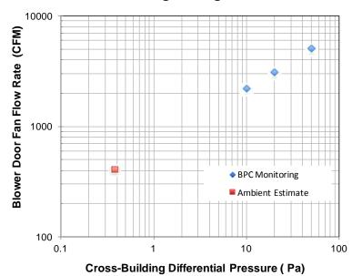
**Building Leakage Curve**
