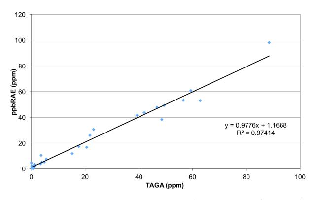
Figure 4: ppbRAE reading versus TAGA mass spectrometer for soil vapor samples (MSRAS, 2006)
