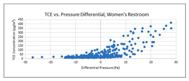
Figure 3: Indoor air TCE versus cross-slab pressure differential (positive values indicate sub-slab region had higher pressure than indoor air) (Reprinted from Hosangadi et al., 2017 with permission John Wiley and Sons)
