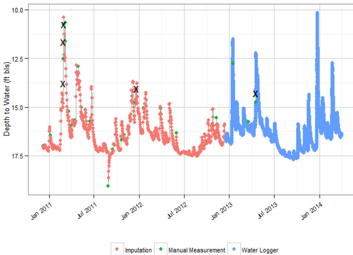
Figure 8-8. Groundwater level measurements used for depth-to-water. “X” indicates where groundwater sample and soil gas sample depth-to-water differ by more than 12 inches.
