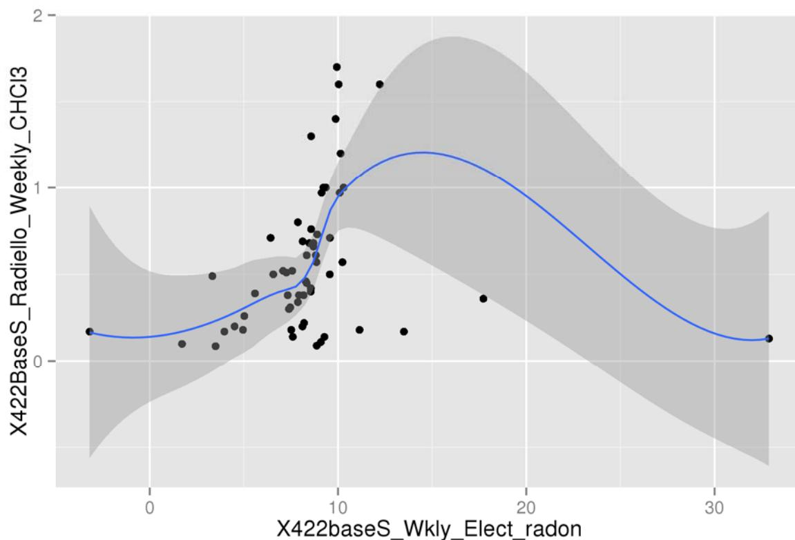
**Figure 6-8. XY plot of radon (pCi/L) vs. chloroform (µg/m<sup>3</sup>), 422 basement south, January 2011 to February 2012 data set.**
