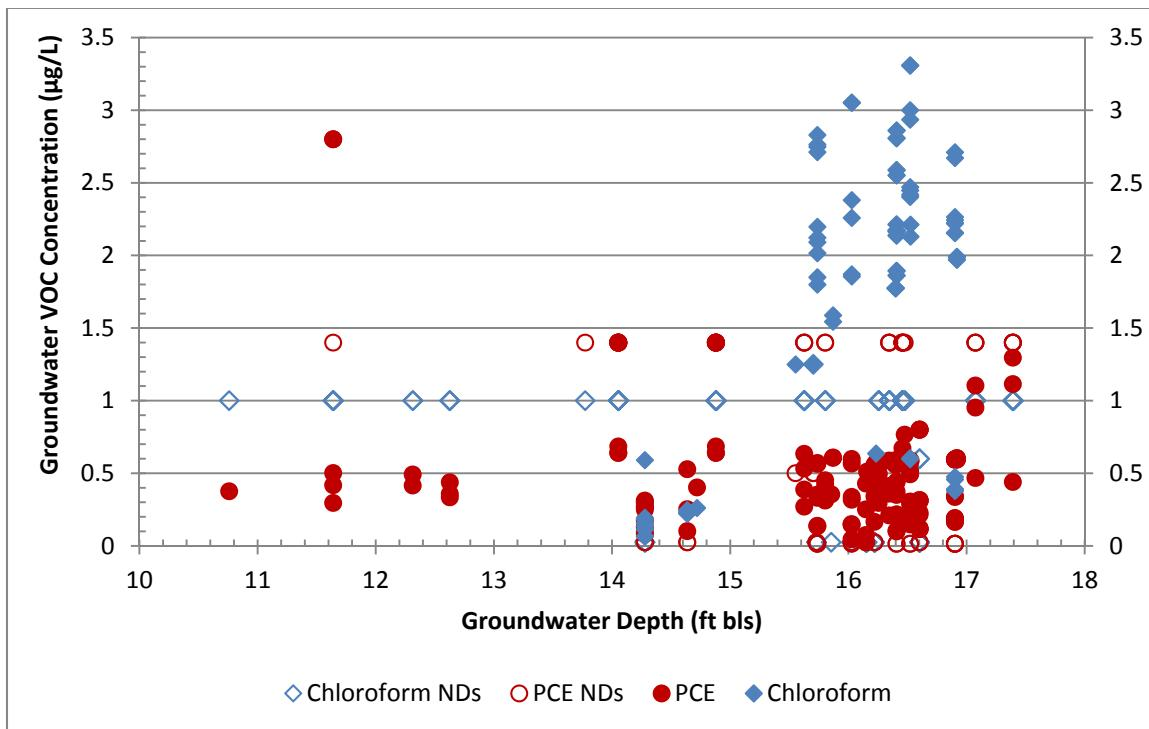
**Figure 8-4. Plot of groundwater PCE and chloroform concentrations against groundwater depth (open symbols are nondetects plotted at one-half the detection limit) (data set over full study period discussed in this report).**
