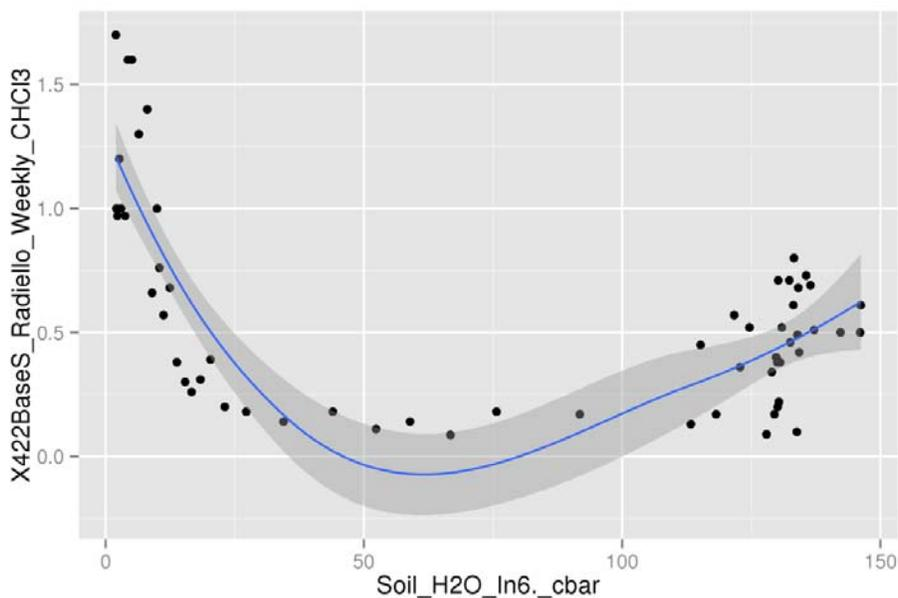
**Figure 6-40. XY plot of soil moisture at 6 ft bls (immediately below floor) vs. chloroform concentration, Radiello samples, January 2011 to February 2012 (includes locally weighted scatterplot smoothing [LOESS] line [blue], with a 95% confidence interval [shaded]).**
