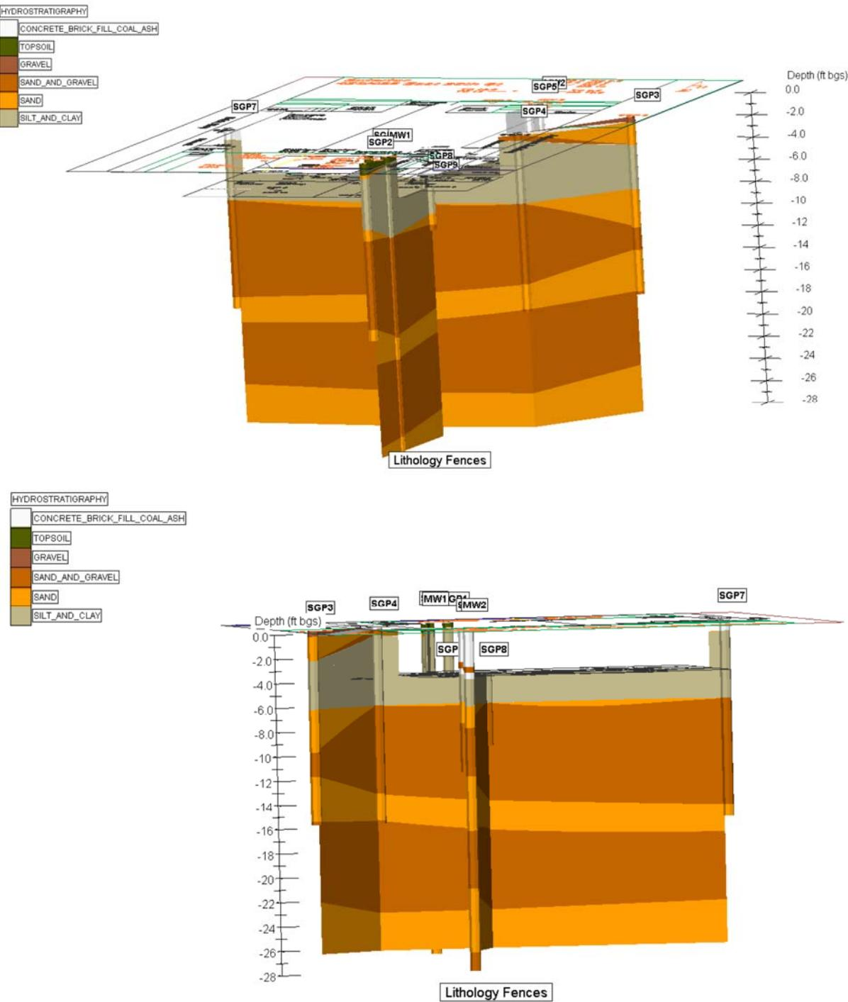
**Figure 3-1.** Lithological fence diagram beneath the 422/420 house, toward N from street (top) and toward S from backyard (bottom). Basement is unshaded with silt and clay (brown) until 6 to 8 ft bls and sand and gravel (burnt orange) and sand (orange) below.
