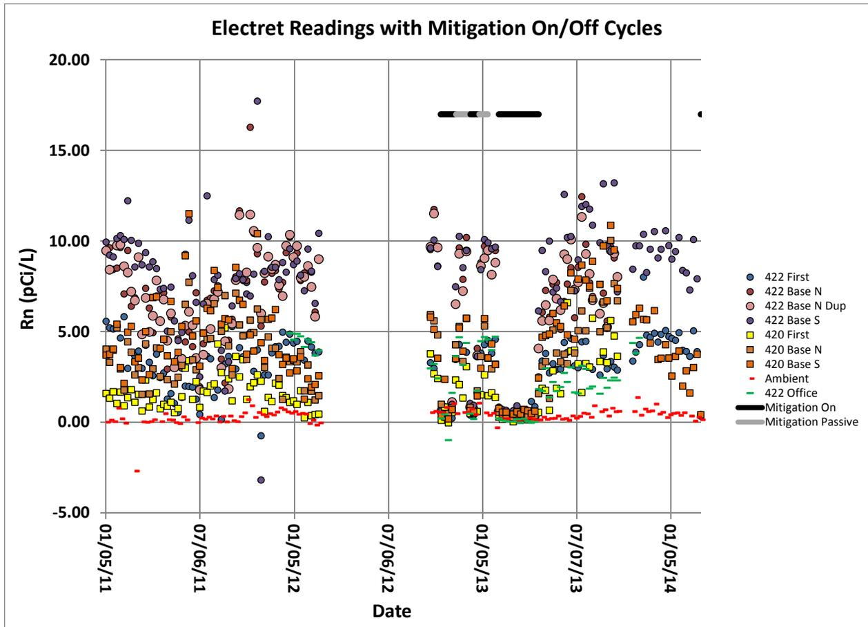
**Figure 5-34. Radon: Weekly time integrated samples (electret).**
