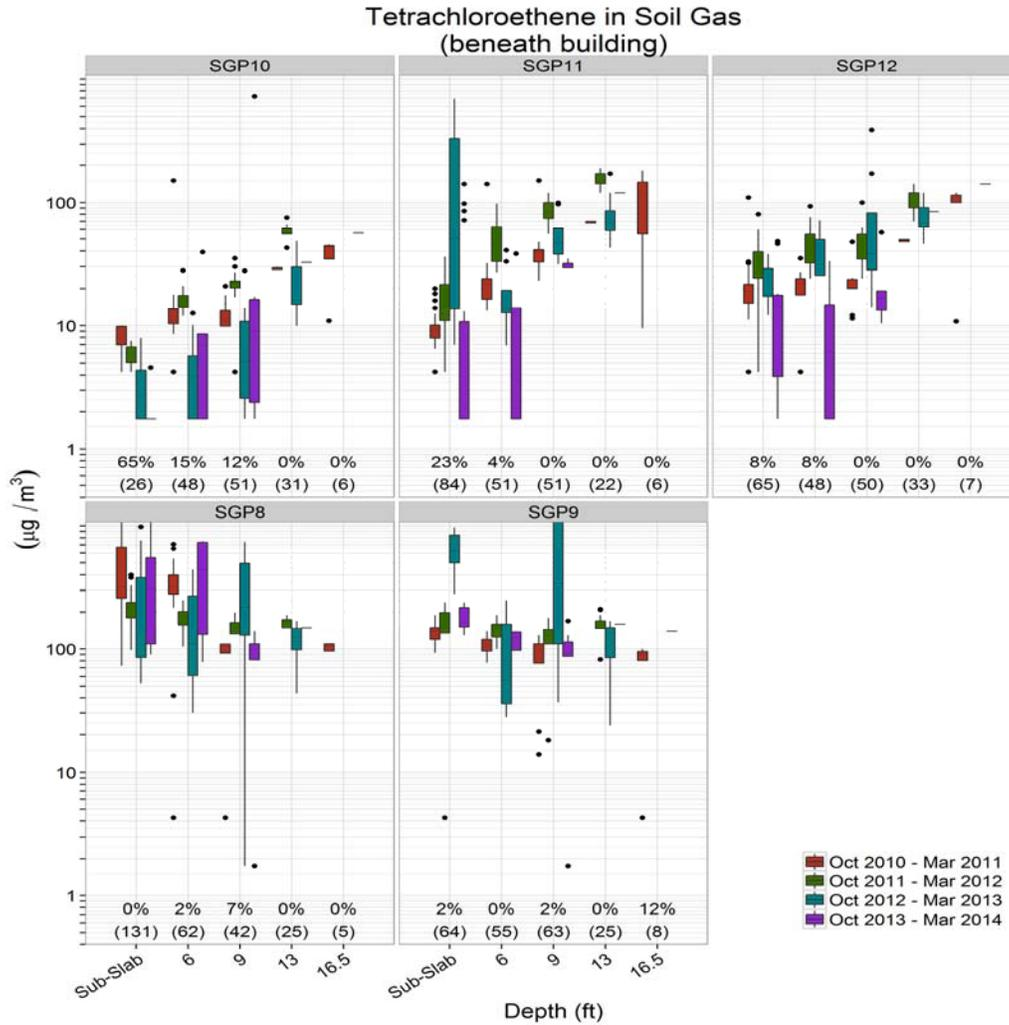
**Figure 7-11. Box and whisker plot for PCE comparing four heating seasons (October to March) interior locations.<sup>a</sup> For each location, five depths are plotted from subslab to 16.5’.**
