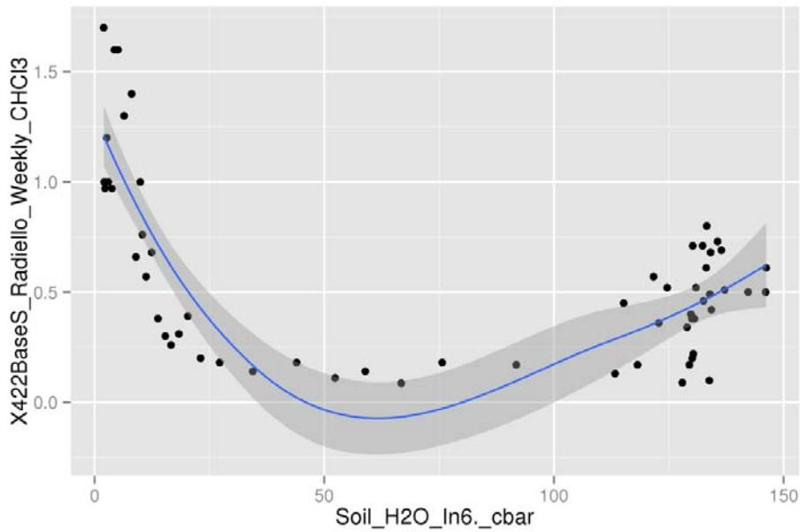
**Figure 6-40.** XY plot of soil moisture at 6 ft bbls (immediately below floor) vs. chloroform concentration, Radiello samples, January 2011 to February 2012 (includes locally weighted scatterplot smoothing [LOESS] line [blue], with a 95% confidence interval [shaded]).
