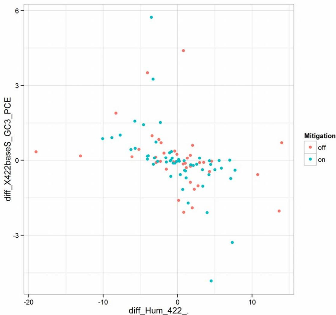
**Figure 6-26. XY graph of first difference in indoor humidity (measured in the 422 2<sup>nd</sup> floor office) vs. first difference in indoor concentration of PCE; online GC data, December 2012 to February 2013.**
