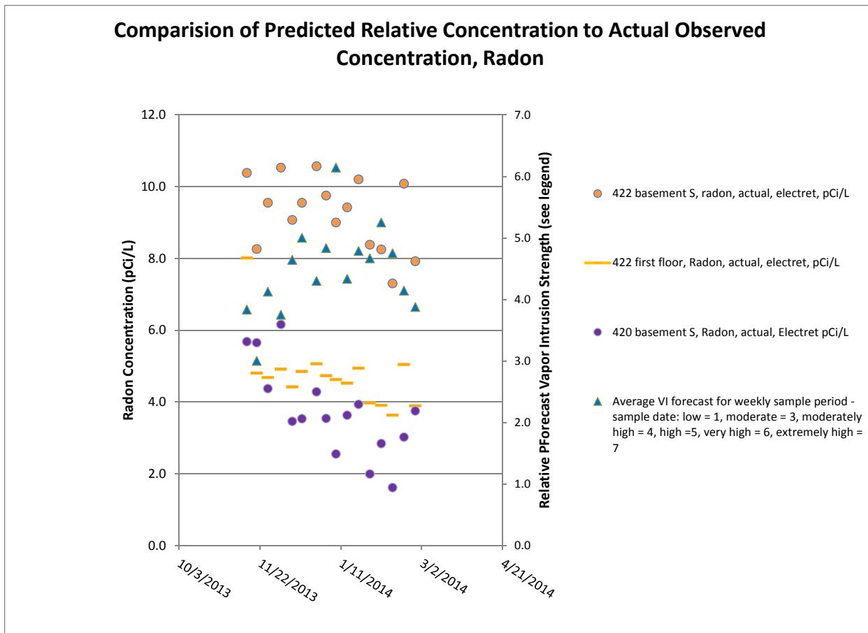
**Figure 7-3. Comparison of predicted concentration to actual observed concentration, radon.**
