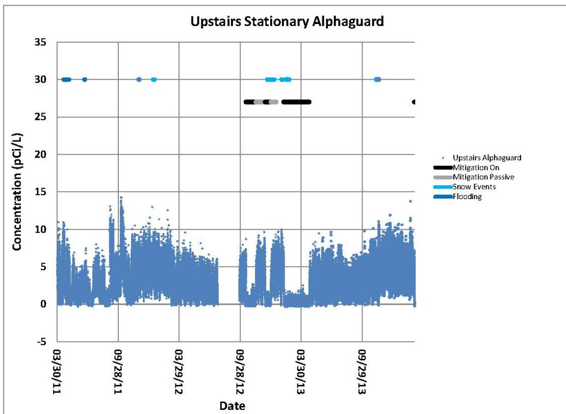
**Figure 5-47. Real-time radon (422, second floor office), 2011–2014.**
