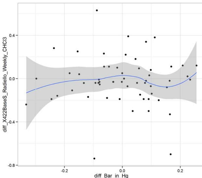
**Figure 6-7b.** XY plot of first difference in barometric pressure vs. first difference chloroform January 2011 to February 2012.
