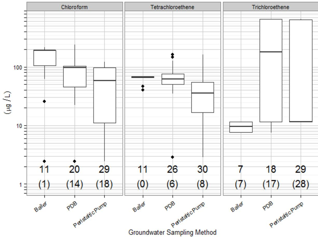
**Figure 8-10. Box and whiskers plots of VOC concentrations in measured in groundwater, organized by sampling method.** Boxes outline 25th and 75th percentiles with heavy bar representing the median (50th percentile) concentration. Number of measurements is given below bars along with the count of nondetects in parentheses.
