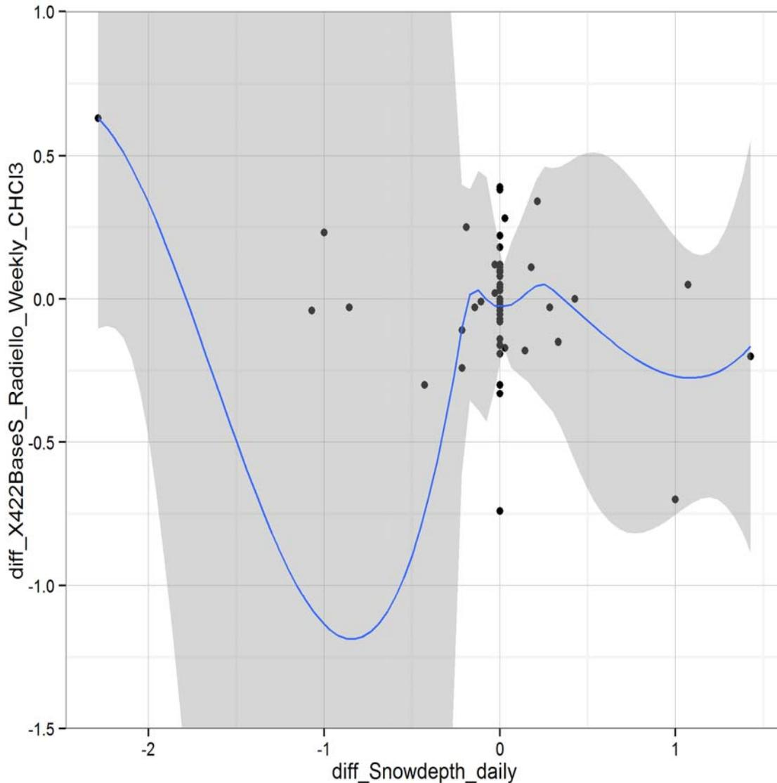
**Figure 6-1. XY plot of first difference in snow depth vs. first difference in chloroform concentration (includes locally weighted scatterplot smoothing [LOESS] line [blue], with a 95% confidence interval [shaded]).**
