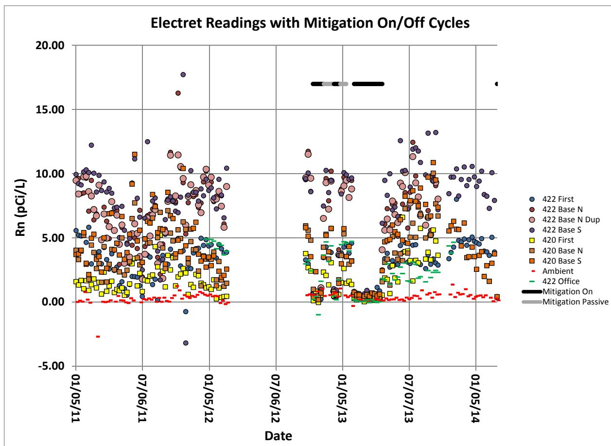
**Figure 5-34. Radon: Weekly time integrated samples (electret).**
