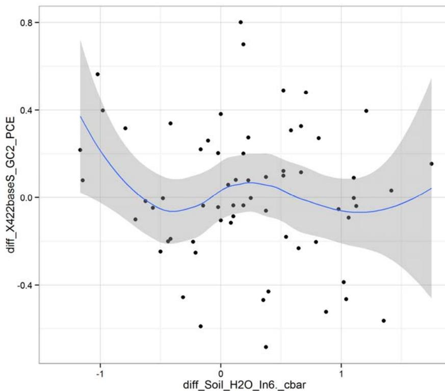
**Figure 6-41. XY plot of first difference of soil moisture at 6 ft bls (immediately below floor) vs. first difference of PCE concentration, online GC measurements, daily aggregation, December 2011 to February 2012 (includes locally weighted scatterplot smoothing [LOESS] line [blue], with a 95% confidence interval [shaded]).**
