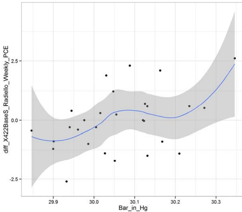
**Figure 6-9. XY plot barometric pressure vs. first difference in PCE concentration.**
