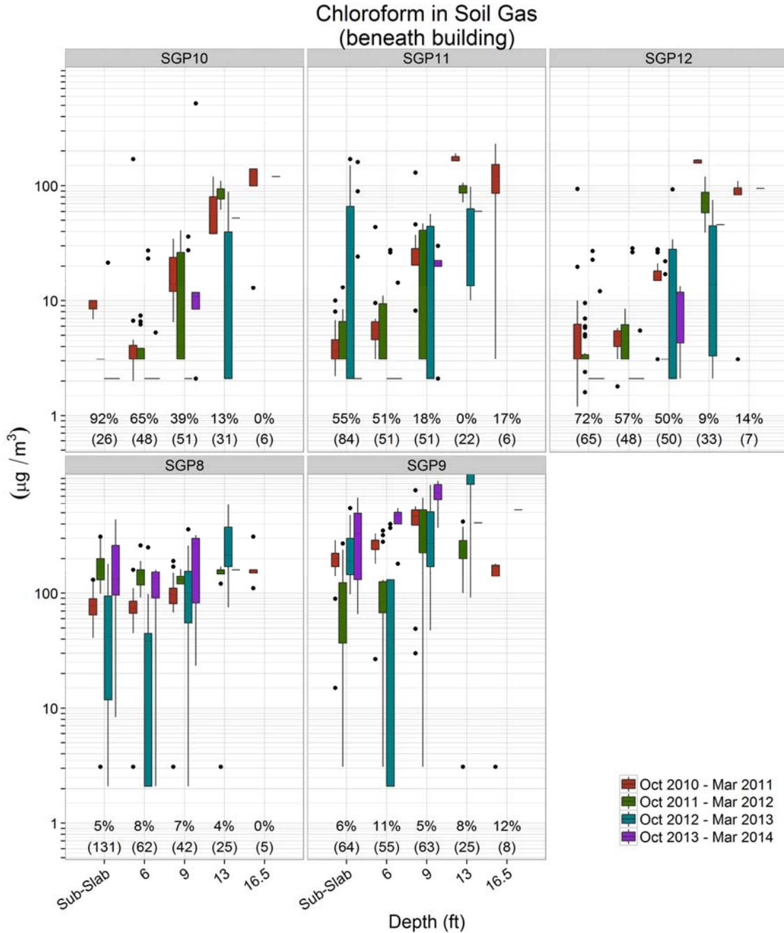
Figure 7-12. Box and whisker plot for chloroform comparing four heating seasons interior locations (October to March) for each location five depths are plotted from subslab to 16.5'.
