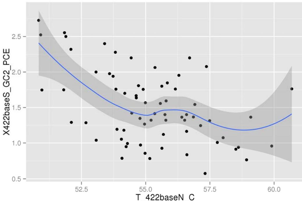
**Figure 6-29.** XY Plot of basement temperature in 422 basement north vs. indoor concentration in 422 basement south, December 2011 to February 2012, on-site GC, daily aggregated data (includes locally weighted scatterplot smoothing [LOESS] line [blue], with a 95% confidence interval [shaded]).
