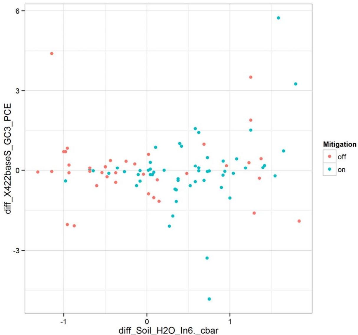
Figure 6-42. XY plot of first difference of soil moisture at 6 ft bsl (immediately below floor) vs. first difference of PCE concentration, online GC measurements, daily aggregation, December 2012 to March 2013.
