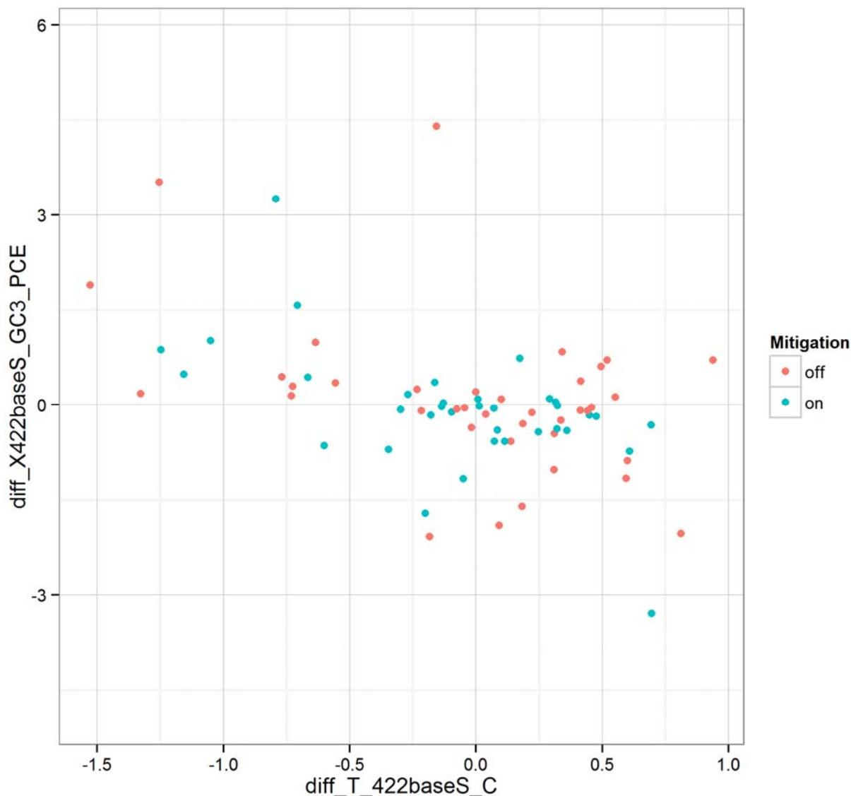
**Figure 6-20. XY plot of the first difference in temperature at the 422 base south location to the first difference in indoor PCE concentration at the same location; online GC data, December 2012 to March 2013.**
