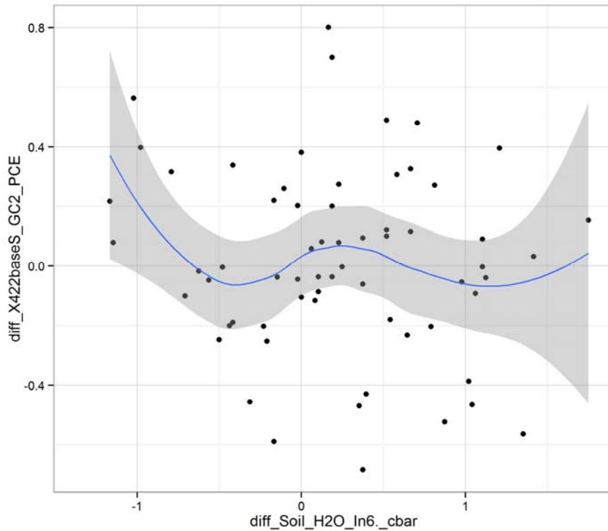
**Figure 6-41.** XY plot of first difference of soil moisture at 6 ft bbls (immediately below floor) vs. first difference of PCE concentration, online GC measurements, daily aggregation, December 2011 to February 2012 (includes locally weighted scatterplot smoothing [LOESS] line [blue], with a 95% confidence interval [shaded]).
