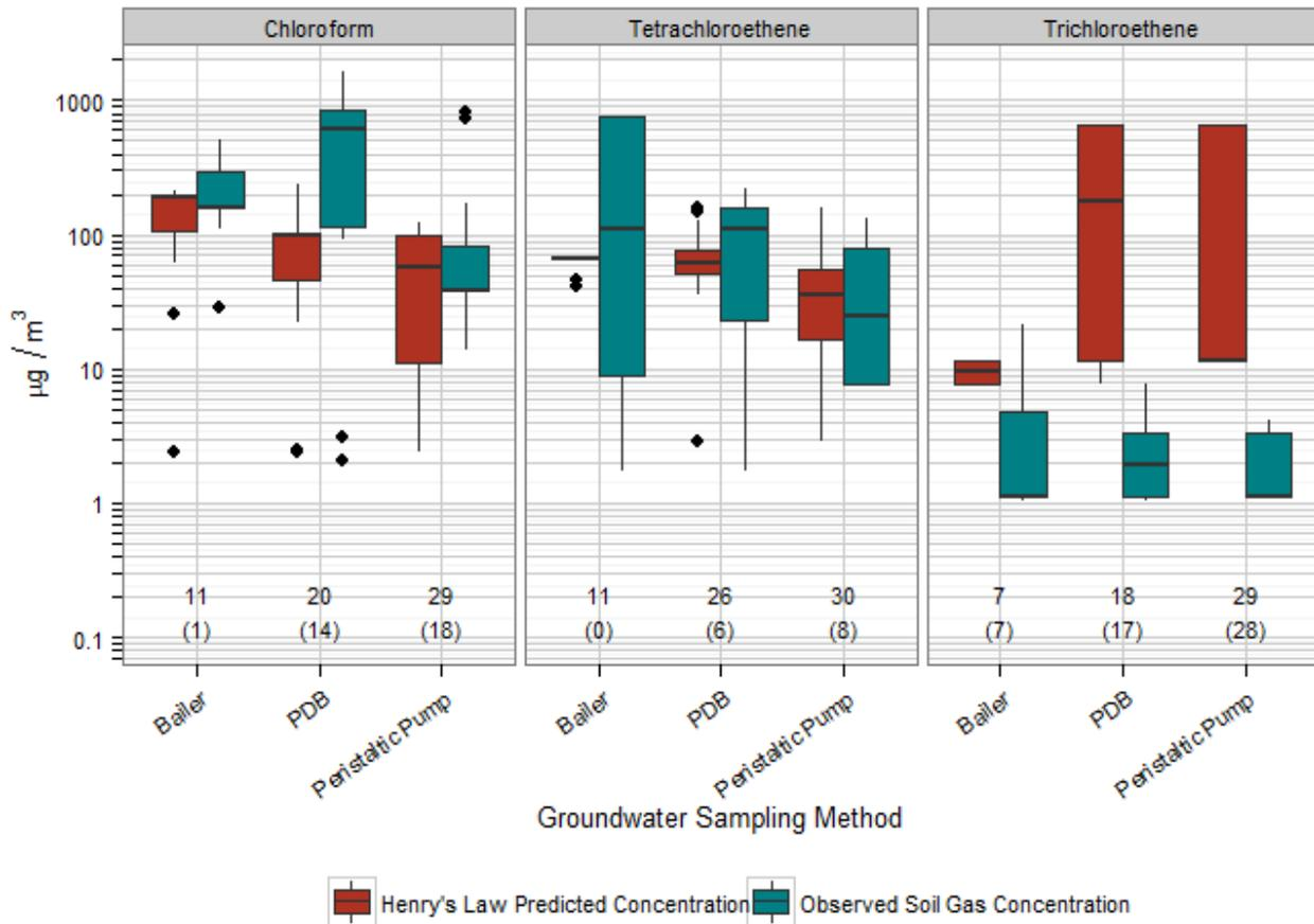
**Figure 8-13. Measured VOC concentrations in groundwater, with the total number of soil gas measurements and number of nondetects below each set of boxes. Each box spans the 25th percentile to 75th percentile range with the median plotted as the bold line.**
