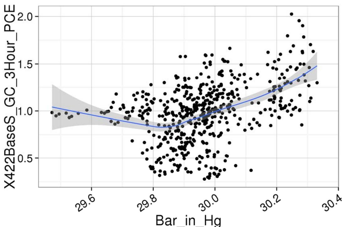
**Figure 6-32. XY plot of barometric pressure vs. PCE, online GC data, 3-hour aggregation, August 2011 to October 2011 (includes locally weighted scatterplot smoothing [LOESS] line [blue], with a 95% confidence interval [shaded]).**
