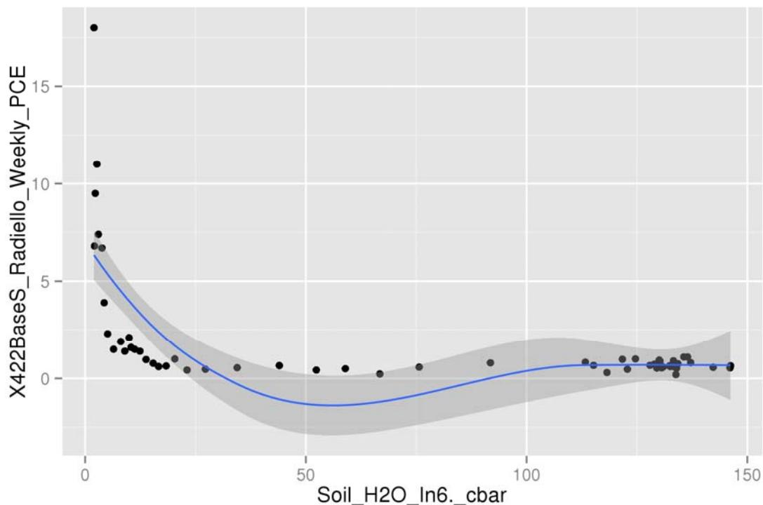
**Figure 6-39.** XY plot of soil moisture at 6 ft bbls (immediately below floor) vs. PCE concentration, Radiello samples, January 2011 to February 2012 (includes locally weighted scatterplot smoothing [LOESS] line [blue], with a 95% confidence interval [shaded]).
