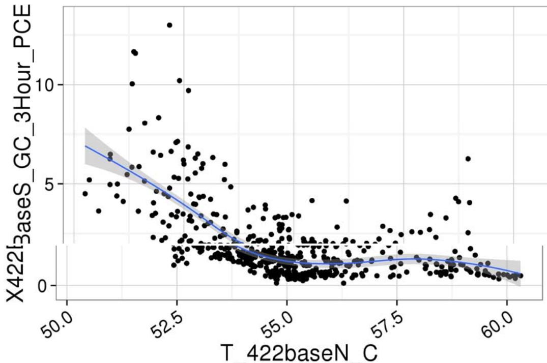
**Figure 6-31.** XY plot of temperature at 422 basement south vs. PCE, 3 hour aggregated data, December 2012 to March 2013 on-site GC (includes locally weighted scatterplot smoothing [LOESS] line [blue], with a 95% confidence interval [shaded]).
