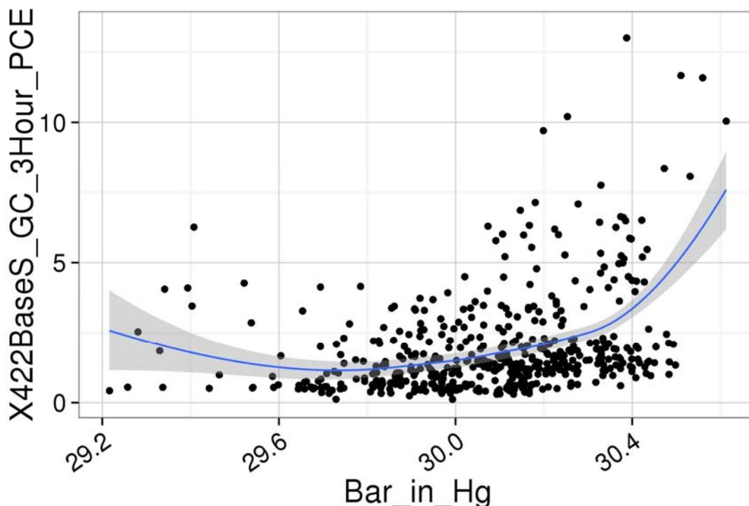
**Figure 6-33. XY plot of barometric pressure vs. PCE, online GC data, 3-hour aggregation; December 2012 to March 2013 (includes locally weighted scatterplot smoothing [LOESS] line [blue], with a 95% confidence interval [shaded]).**
