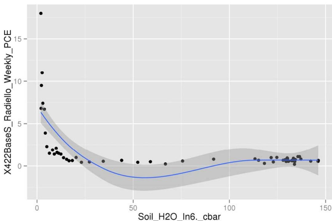
**Figure 6-39. XY plot of soil moisture at 6 ft bls (immediately below floor) vs. PCE concentration, Radiello samples, January 2011 to February 2012 (includes locally weighted scatterplot smoothing [LOESS] line [blue], with a 95% confidence interval [shaded]).**
