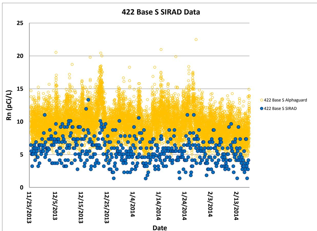
Figure 5-48. Real-time radon (422 south basement) AlphaGUARD vs. SIRAD.
