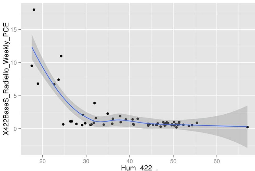
**Figure 6-34. XY plot of indoor humidity (422 office) vs. PCE concentration in 422 basement south; January 2011 to February 2012, Radiello passive sampler data (includes locally weighted scatterplot smoothing [LOESS] line [blue], with a 95% confidence interval [shaded]).**
