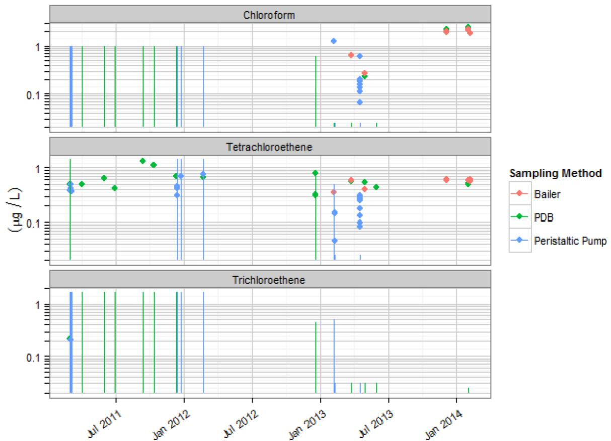
**Figure 8-9. Measured VOC concentrations in groundwater by time and sampling method (vertical lines indicate nondetects plotted from zero to one-half the detection limit).**
