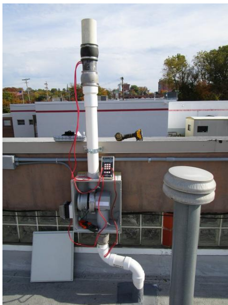
Figure 8: Measuring System Airflow & Amperage
