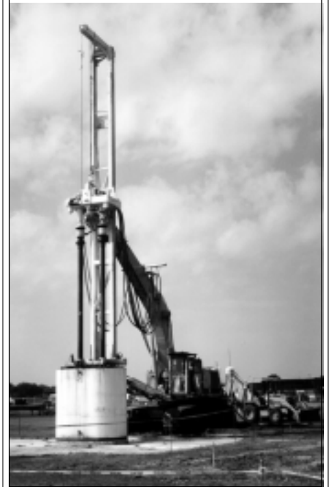
Figure 1: Rotary Steam Stripping at the Pinellas Plant
