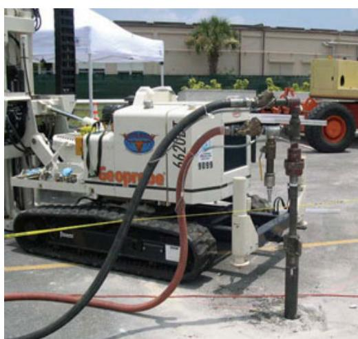
**Figure 2.** Pneumatic and product hoses attached to a 360°-rotatable injection nozzle on a direct push rig.
