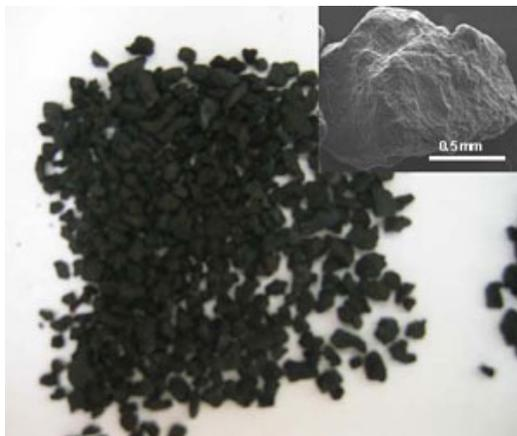
**Figure 1.** RAC consisting of Fe/Pd on GAC.
