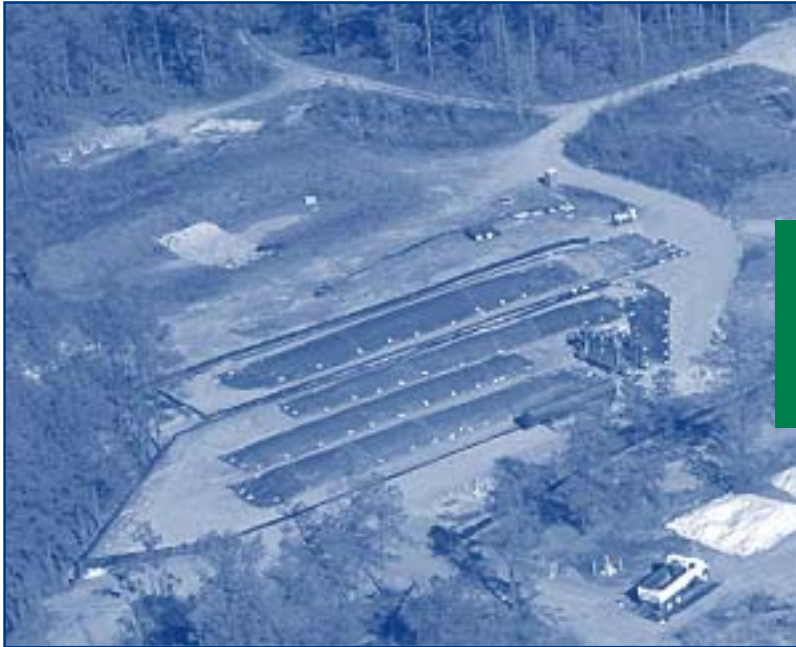
Figure 2. Recent treatability studies on soil bioremediation at the SRS CMP Pits waste site evaluated various combinations of soil amendment applied through windrowing.
