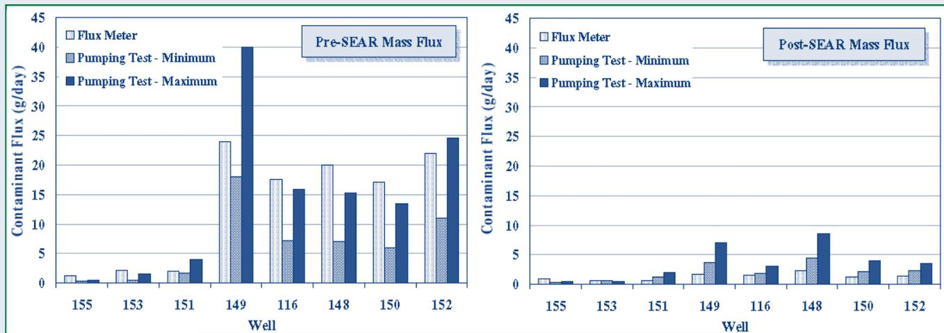
*Figure 3. Compiled data collected through both the flux meter and integral pumping techniques show similarly significant reductions in mass flux at OU2 as a result of SEAR application.*
