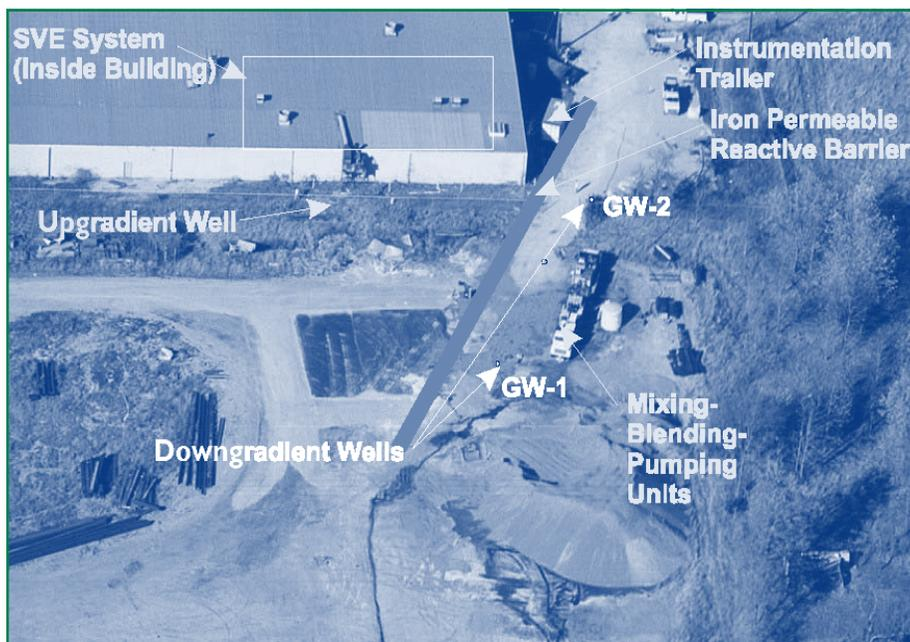
*Figure 2. The PRB spans 240 feet along a path intercepting ground-water flow from the contaminant source, which is located directly beneath a building currently housing the SVE system.*
