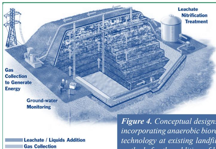
**Figure 4.** Conceptual designs for incorporating anaerobic bioreactor-based technology at existing landfills involve methods for the addition of liquids as well as the recirculation of leachate.
