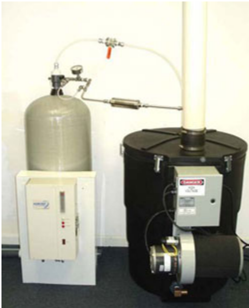
Figure 1. Single in-line water treatment system involving both ozone/perozone injection and air stripping technologies.
