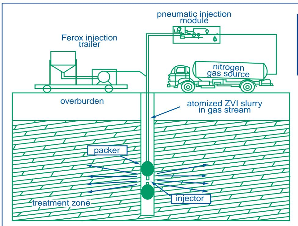
**Figure 3.** The injected Ferox<sup>SM</sup> process slurry produces a fine mist that disperses iron powder within the subsurface.
