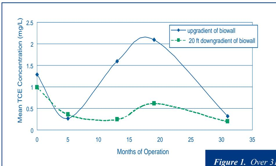
Figure 1. Over 31 months of treatment at Offutt AFB, the mean TCE removal was approximately 70%.
