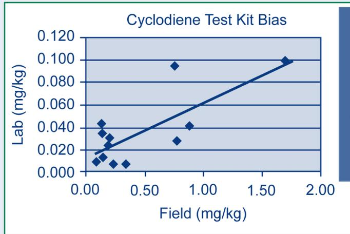
Figure 4. Positive bias was observed in the cyclodiene test kit results obtained in the field at the East Palo Alto pesticide-contaminated area.
