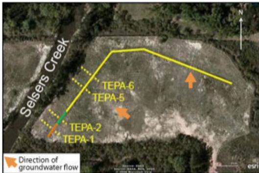
**Figure 2.** Configuration of PRB system at the Delatte Metals site showing locations of transects sampled; orange segment represents former pilot-scale PRB containing 1:1:1 cow manure, wood chips, and limestone gravel, and green segment represents former pilot-scale PRB containing 2:1 cow manure and limestone (as used in full-scale PRB depicted in yellow).
