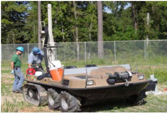
**Figure 1.** GeoProbe® deployment on a swamp buggy to install monitoring wells.
