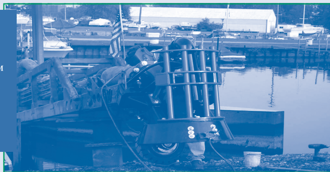
Figure 2. The 8-inch hydraulic dredge with attached Vic-Vac ™ prepares to launch in target portions of the Ashtabula River AOC.
