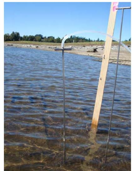
Figure 5. Sample collection in sub-armor of the sediment cap at the McCormick & Baxter site.
