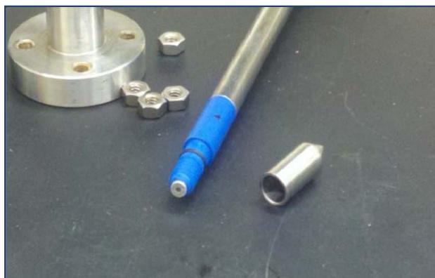
Figure 1. Acoustic probe tip and microphone embedded in the Delrin isolator.
