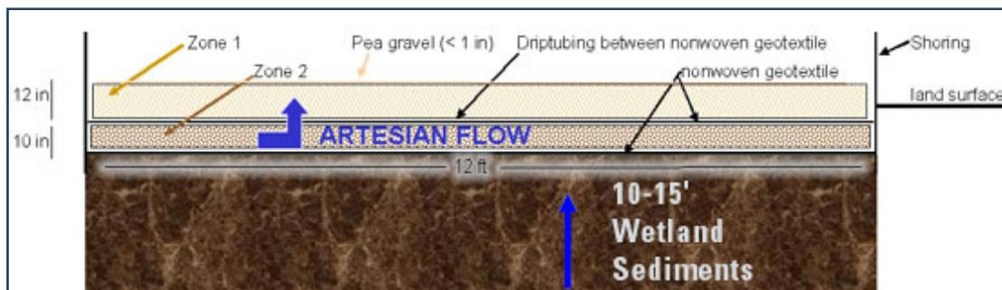
Figure 2. Reactive biomat at APG with a bioaugmented upper organic zone and a lower zone designed to enhance abiotic degradation of contaminants.
