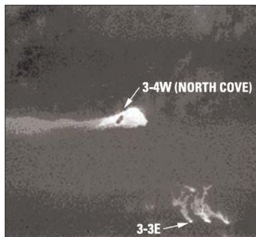
*Figure 5. Thermal infrared imagery showing the temperature disparity between two groundwater seep areas and the surrounding environment. The reactive mat was installed on the surface of seep 3-4W.*
