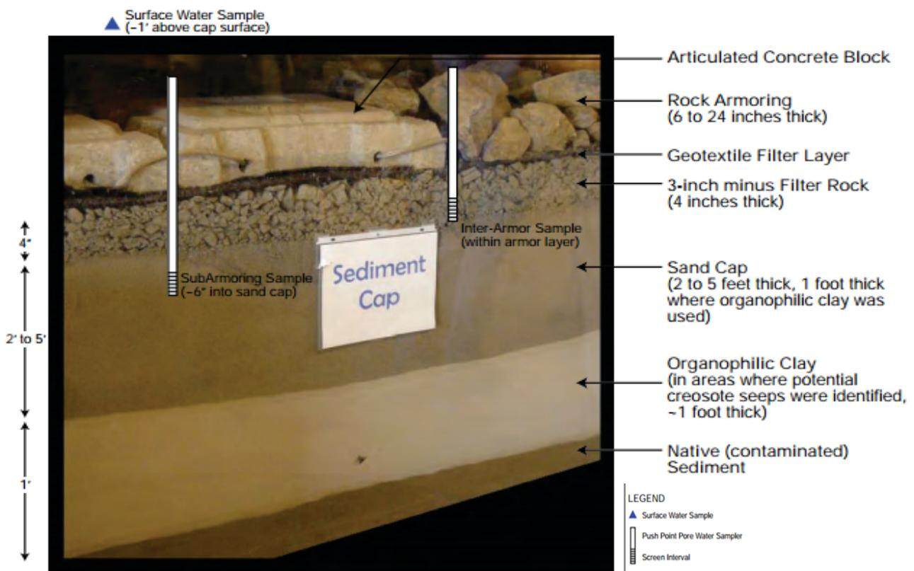
Figure 3. Cross-section of sediment cap installed at the McCormick & Baxter site.
