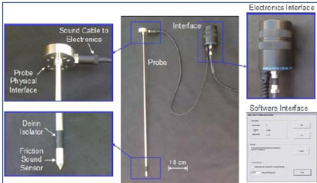
Figure 2. Commercial prototype SED-FSP setup
