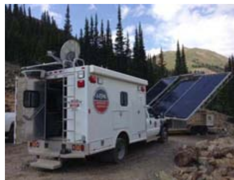
Figure 1. Solar energy equipment supporting remedy construction at the Pennsylvania Mine.
