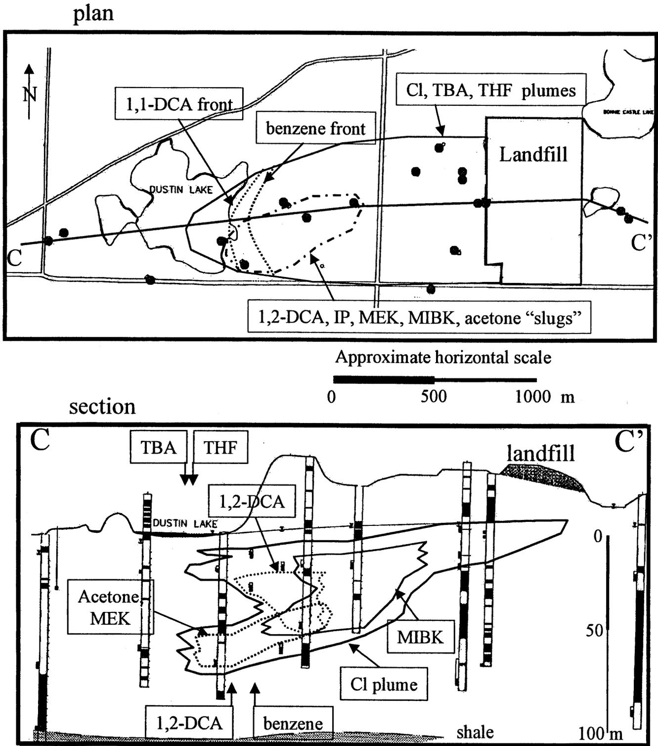
Figure 1. Plan and cross section showing the landfill, monitoring wells, basic hydrostratigraphy (dark units are aquitards), and approximate extent of the various chemical plumes.
