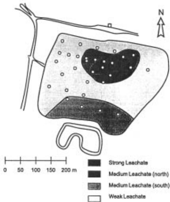
Figure 2. Division of the landfill into four areas with different leachate (Kjeldsen et al., 1998a).
