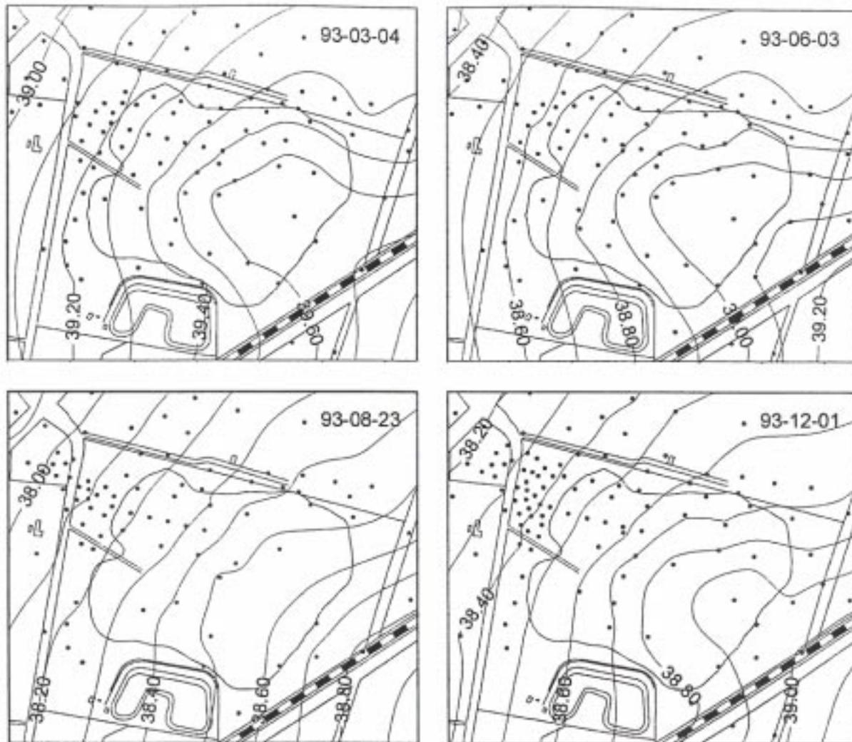
**Figure 3.** Mounding of the leachate-groundwater table below Grindsted Landfill shown as isopotential contours for the landfill and surrounding area at 4 different seasons during 1993. Modified from Kjeldsen et al. (1998).
