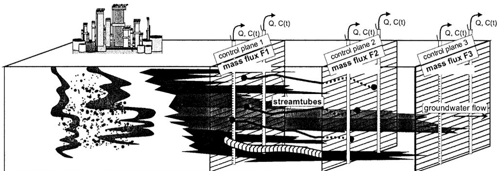
**Figure 6.** With the new site evaluation technique, rather than estimating the contaminant distribution based on point-concentrations, the entire contaminant mass flux (immission) across given control planes is quantified.
