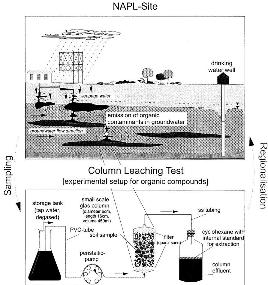
**Figure 2.** The emission from a contaminated site (location, size and strength of source) is commonly performed on the basis of *soil sampling* and *leaching tests*. Even though the leaching test procedures are being improved considerably and also standardised, the regionalisation of the test results is considered highly uncertain.
