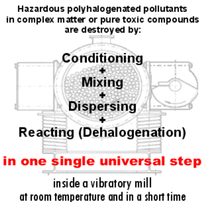
Figure 1 and 2: Overview of the DMCR process characterization: One example outlined (rough, simplified scheme, not stoichiometric) for dehalogenation using DMCR: PCBs are dehalogenated by Magnesium metal in the presence of an appropriate hydrogen donor (alcohols, polyethers, amines and so forth) yielding harmless biphenyl and magnesium chloride [6].
