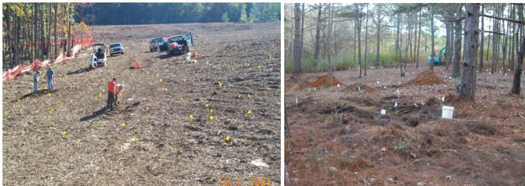
Figure 3-5. Mag-and-flag survey (left) and flags placed following a mag-and-flag survey (right) (Photos courtesy of Tetra Tech EC, Inc.).
