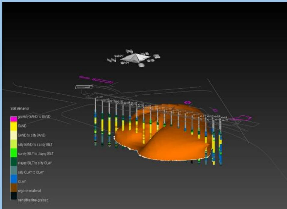
*Figure 6. 3-D Visualization Component of Remediation/Mitigation CSM. The Remediation/Mitigation CSM enhances a project team's ability to evaluate and modify remedial designs during implementation to minimize resources and maximize remedy effectiveness.*
