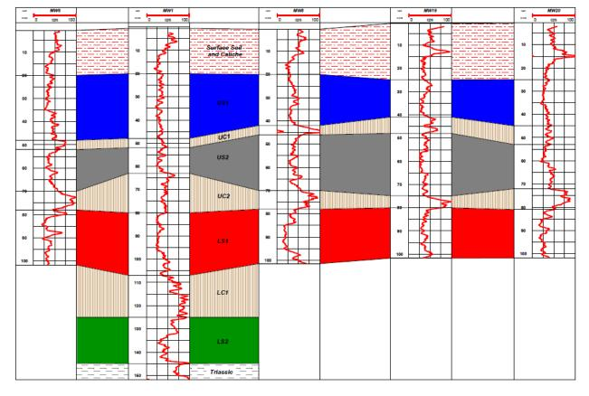
The dissolved-phase plume is present in US2 (saturated at the time of the optimization review) and LS1. Contaminants are transported in the subsurface in both the dissolved phase and vapor phase. Existing private water supply wells are not typically grouted above the screened interval, or have long
