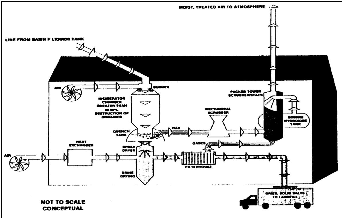
Figure 1. Conceptual Schematic of the Submerged Quench Incineration System (prepared by Woodward-Clyde Consultants)
