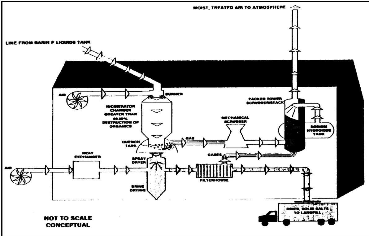
*Figure 1. Conceptual Schematic of the Submerged Quench Incineration System
