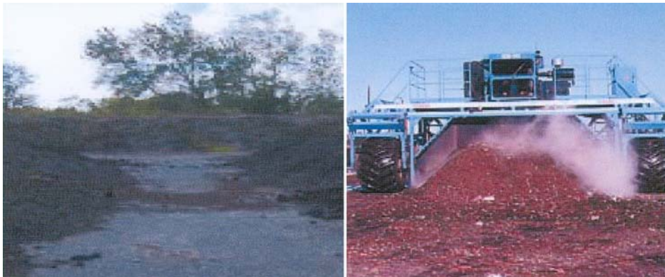
Figure 11: Piles of finished compost (left) and the turning of windrows at Fresh Kills compost facility
