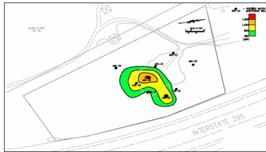
Figure 6. Two-Week Post Injection NAPL Plume
