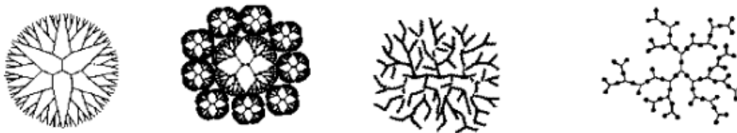
Figure 4. Different dendritic polymers: dendrimer, core-shell tecto(dendrimer), dendrigraft polymer, hyperbranched polymer (Diallo 2005)
