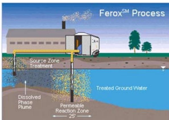
**Figure 6: NZVI Dispersion Via Injection.** An open borehole or direct-push injector assembly casing is used to position the downhole apparatus into the subsurface. Once in place, zero-valent iron powder is injected into the formation as a slurry or as a dry material. Nitrogen gas or compressed air is used as the carrier fluid (ARS Ferox Technology, 2009).
