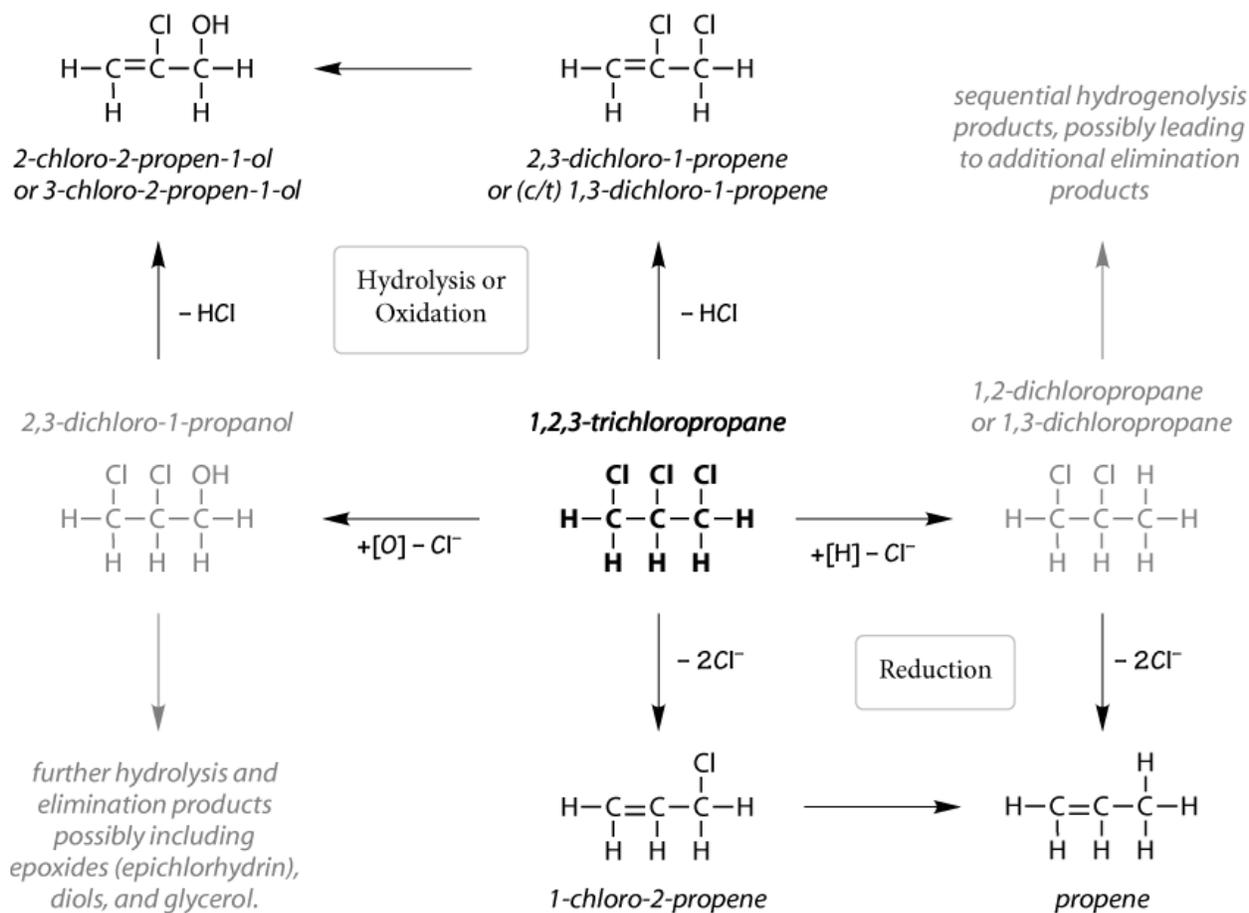
**Figure 3. Anticipated Primary Reaction Pathways for Degradation of TCP.** Oxidation, hydrolysis, and hydrogenolysis are represented by the horizontal arrows. Elimination (dehydrochlorination) and reductive elimination (reductive  $\text{e}^-$ -elimination) are shown with vertical arrows. [O] represents oxygenation (by oxidation or hydrolysis), [H] represents reduction. Gray indicates products that are likely to be of lesser significance (Tratnyek and Sarathy, 2008).
