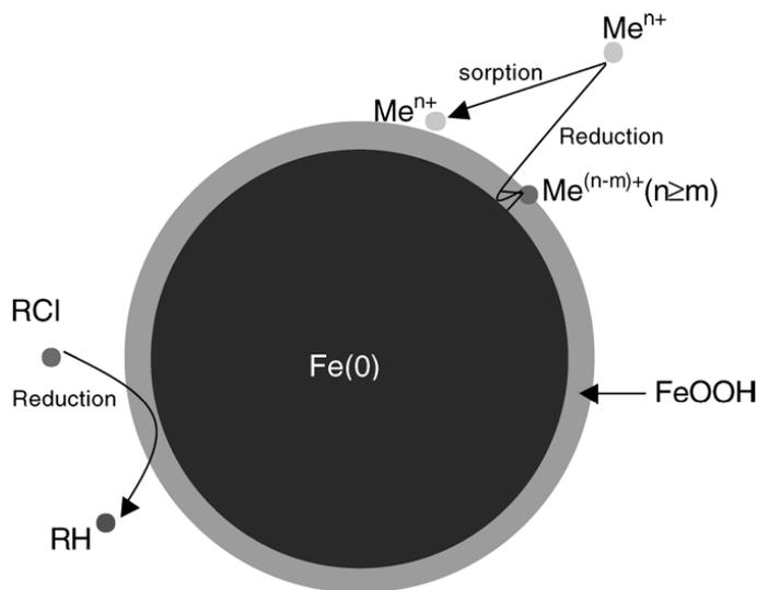
**Figure 1: The Core-Shell Model of Zero-Valent Iron Nanoparticles.** The core consists of mainly zero-valent iron and provides the reducing power for reactions with environmental contaminants. The shell is largely iron oxides/hydroxides formed from the oxidation of zero-valent iron. The shell provides sites for chemical complex formation (*e.g.*, chemisorption) (Li, Elliot, and Zhang, 2006).
