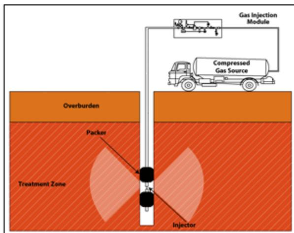
**Figure 7: Pneumatic Fracturing.** Pneumatic fracturing can best be described as a process whereby a gas is injected into the subsurface at pressures exceeding the natural *in situ* pressures present in the soil / rock interface (i.e., overburden pressure, cohesive stresses, etc.) and at flow volumes exceeding the natural permeability of the subsurface (ARS Ferox Technology, 2009).
