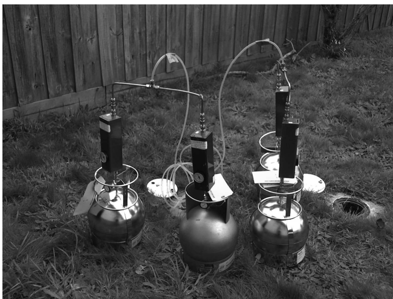
Figure 1: Soil vapour sampling using summa canisters.
