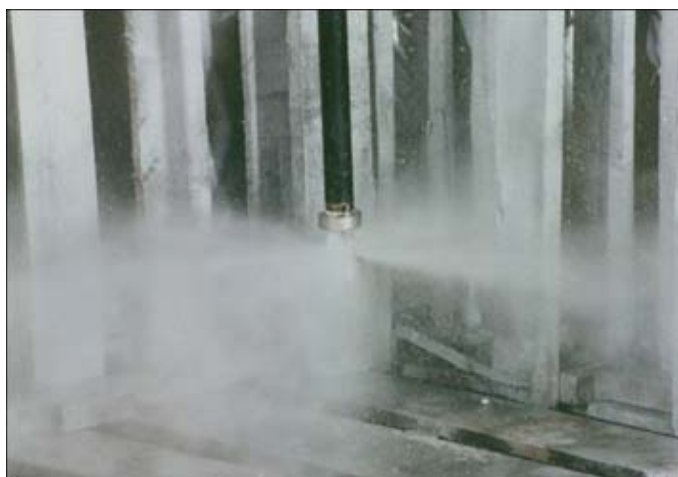
Figure 8: Liquid Atomization Injection. Liquid atomization injection (LAI) is a very effective method for injecting liquids uniformly within all types of geology. In addition, injection radii of influence are considerably greater than that achievable using conventional hydraulic injection. LAI relies upon the premise that it is more effective to inject gases or “aerosols” into the subsurface than it is to inject an incompressible liquid into the subsurface (ARS Ferox Technology, accessed July 8, 2009).
