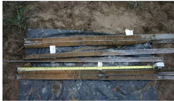
**FIGURE 10. Evidence (black striping) of thorough BOS 100<sup>®</sup> distribution.**
