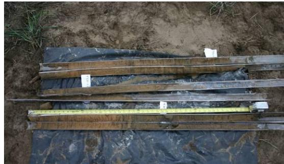
**FIGURE 10. Evidence (black striping) of thorough BOS 100® distribution.**
