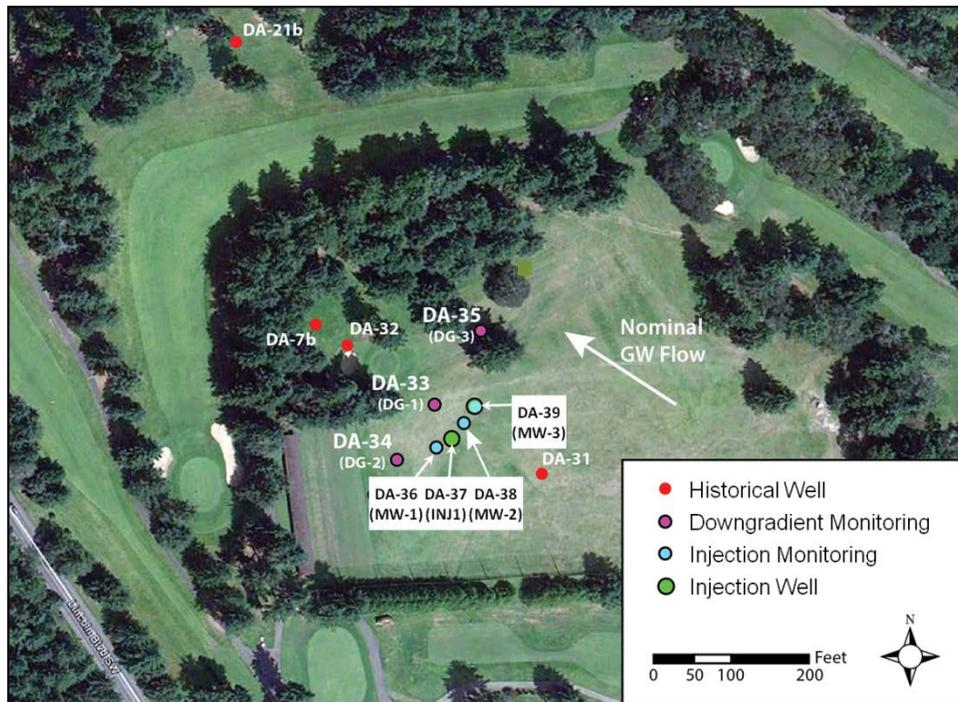
**Figure 5. Site map showing existing wells at the test site (prior to the start of the current demonstration project).**
