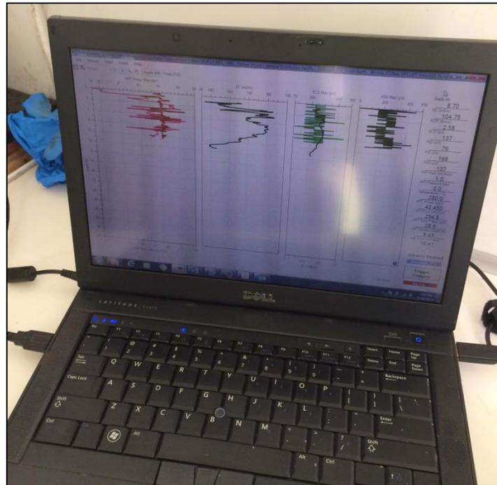
Photo 2: Real-time HPT data reading.
