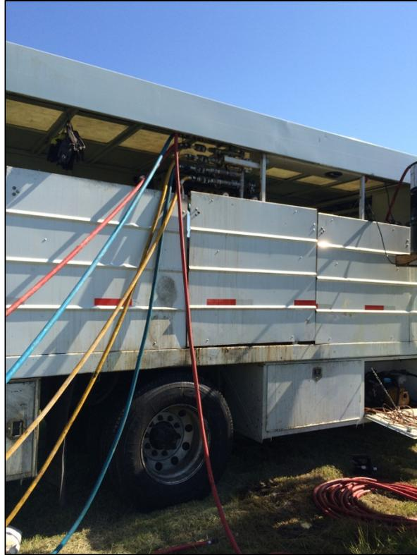
Photo 13: Hoses connected to injection manifold in trailer.
