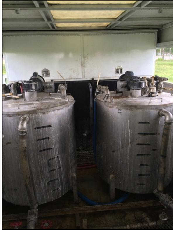
Photo 9: EHC-L mixing tanks in the injection trailer.
