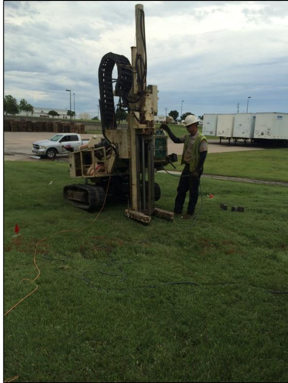
Photo 3: HPT drilling rig.
