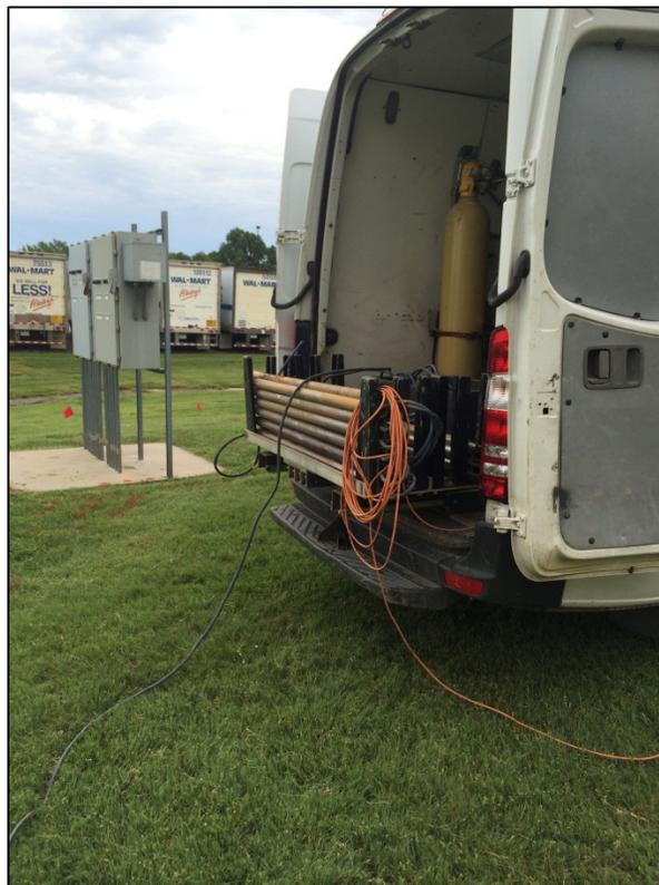
Photo 4: HPT trailer with cables in the HPT rod shown.
