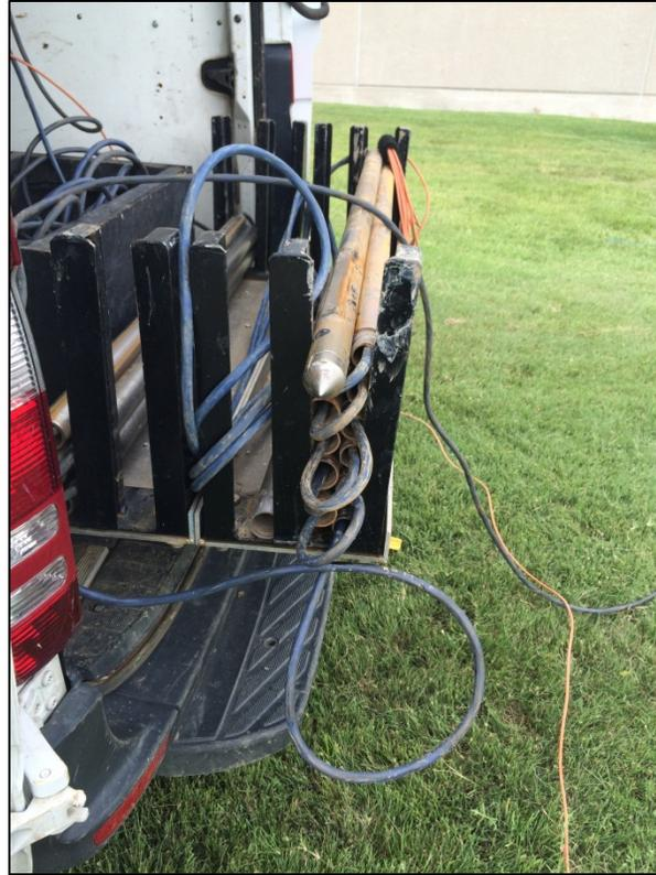
Photo 5: Close up of the HPT injection tip and cables.
