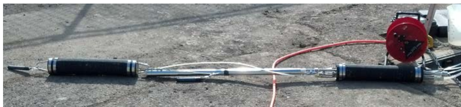
Figure 5. Typical Straddle-Packer Setup. Includes a bladder pump suspended between the packers to sample the target fracture zone interval. Tubing associated with bladder pump operation and inflation of the bottom packer, are passed through the top packer using air-tight stainless steel tubes designed and manufactured into the packer.
