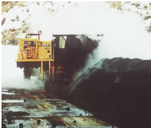
Figure 12. Steam Rising From Compost During Tilling
