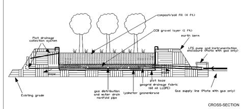
Each study plot consists of a gas distribution plenum (sandy-gravel) covered with a bioreactive layer of landfill cover soil mixed with compost. Lysimeters installed in each study plot are designed to capture infiltrating precipitation. Infiltrating precipitation is conveyed to water meters to measure volumes over time. A sub-base gravel mixture has been spread to form the base of each research plot. Landfill gas distribution piping is embedded into the base mixture
