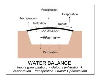
Landfill capping systems reduce the quantity of water moving into and through underlying wastes. Water movement through the organic waste matrix creates leachate, and can result in contamination of ground water and surface water. The effectiveness of a can design is based on the classical water balance equation based on the principle of conservation of mass.
