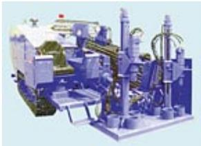
All directional drilling rigs have a few common characteristics: a capacity for using a fluid while drilling and a method for providing a thrust force to the drill string to compensate for lost weight on the bit when drilling the horizontal section of a borehole.
