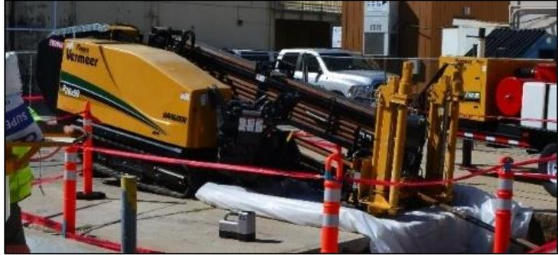
**Figure 2. Common Directional Drilling Rig**
