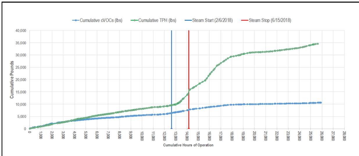
**Figure 8. Contaminant Recovery Results at Building 379, NASNI, California**
